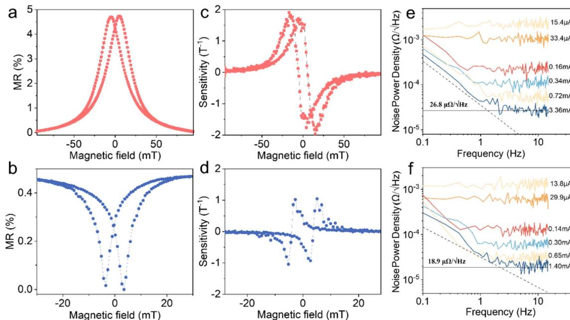
Fig. 2 Magneto-electric performance of printed magneto-resistive sensors. (a) MR, (c) sensitivity and (e) noise of the printed sensor with  $[\text{Co}/\text{Cu}]_{50}$  GMR microflakes as functional fillers. (b) MR, (d) sensitivity and (f) noise of the printed sensor with  $\text{Ni}_{97}\text{Co}_3$  AMR microparticles as functional fillers. All measurements are performed at room temperature.
