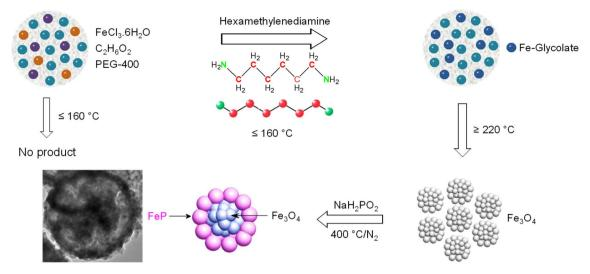
Scheme 1 Schematic summarizing the different steps involved in the preparation of FeP/Fe<sub>3</sub>O<sub>4</sub>
