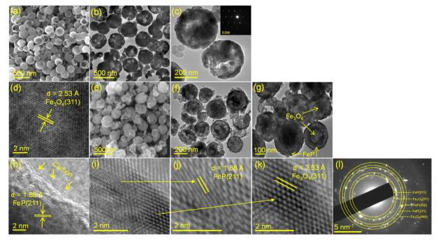
Fig. 3 FESEM and TEM/HRTEM images of Fe<sub>3</sub>O<sub>4</sub> (a-d) and FeP/Fe<sub>3</sub>O<sub>4</sub> (e-k), and SAED patterns of FeP/Fe<sub>3</sub>O<sub>4</sub> (I).
