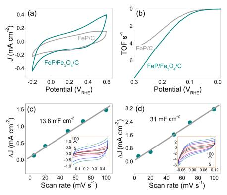
Fig. 6 CVs (a) and TOF profiles (b), plots of the current density (and CVs, inset figure) of FeP/C (c) and FeP/Fe<sub>3</sub>O<sub>4</sub>/C (d) vs. the scan rate.
