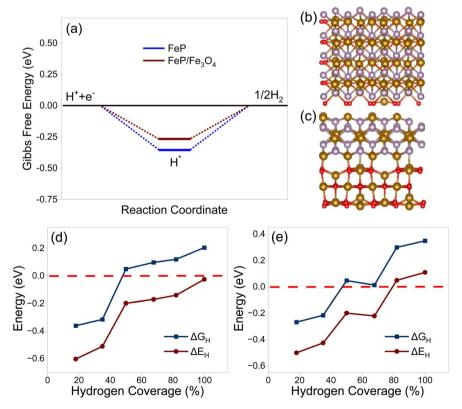
Fig. 9 (a) Free-energy diagram for the HER on bare FeP and FeP/Fe<sub>3</sub>O<sub>4</sub> surfaces, (b) top and (c) side views of hydrogen adsorption. The relationship between the differential adsorption energy ( $\Delta E_{\rm H}$ ), adsorption free energy ( $\Delta G_{\rm H}$ ), and hydrogen coverage on the (d) FeP surface and (e) FeP/Fe<sub>3</sub>O<sub>4</sub> composite layer.
