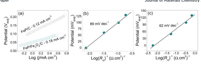
Exchange current density (a) and Tafel slopes of FeP/C (b) and FeP/Fe<sub>3</sub>O<sub>4</sub>/C (c).
