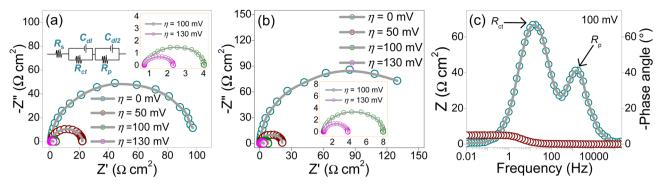
Fig. 7 Nyquist plots of (a) FeP/C and (b) FeP/Fe<sub>3</sub>O<sub>4</sub>/C, and (c) Bode plot of FeP/Fe<sub>3</sub>O<sub>4</sub>/C.
