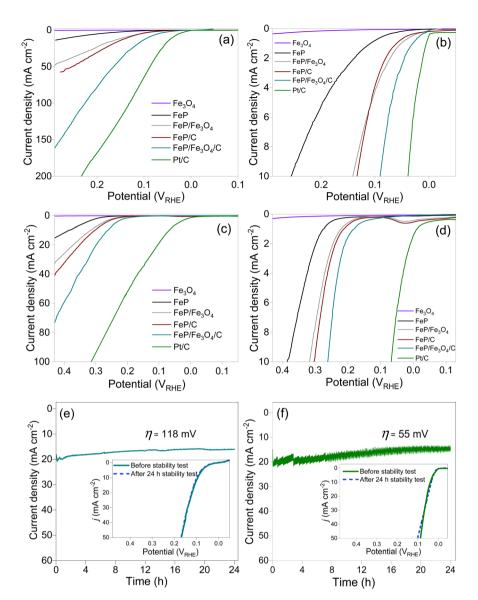
Fig. 4 Polarization curves of Fe<sub>3</sub>O<sub>4</sub>, FeP, FeP/Fe<sub>3</sub>O<sub>4</sub>, carbon-supported FeP and FeP/Fe<sub>3</sub>O<sub>4</sub>, and Pt/C in acidic (a and b) and basic (c and d) media. Current-time profile and polarization curves (figure inset) recorded before and after stability tests of the FeP/Fe<sub>3</sub>O<sub>4</sub>/C (e) and commercial Pt/C (f). Stability was evaluated in 0.5 M H<sub>2</sub>SO<sub>4</sub> aqueous solution.
