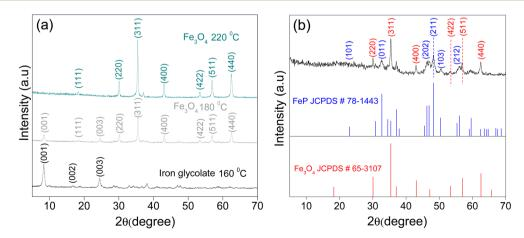
Fig. 1 XRD patterns showing the (a) temperature-dependent evolution of iron glycolate into Fe<sub>3</sub>O<sub>4</sub>, and (b) transformation of Fe<sub>3</sub>O<sub>4</sub> into FeP/ Fe<sub>3</sub>O<sub>4</sub> after phosphidation.
