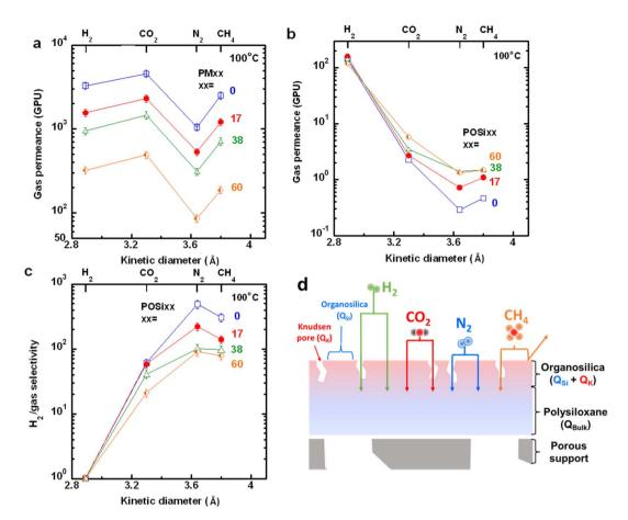
Fig. 4 Pure-gas transport properties of PM and POSi membranes at 100 °C. Comparison of gas permeance in (a) PM and (b) POSi membranes. (c) H<sub>2</sub>/gas selectivity of POSi membranes. (d) Schematic of a series-parallel flow model in POSi membranes.
