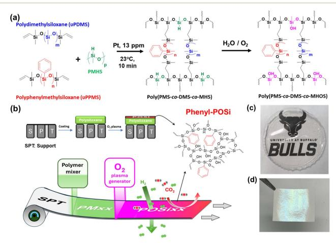
Fig. 1 Our synthesis approach to POSi membranes (POSixx) derived from poly(PMS-co-DMS-co-MHOS). (a) Synthesis of poly(PMS-co-DMS-co-MHOS) by hydrosilylation reaction followed by hydrolysis and oxidation of the unreacted Si-H groups. (b) Preparation of POSi membranes, including fabrication of polysiloxane TFC membranes (PMxx) and oxygen plasma treatment. Photos of (c) a freestanding polysiloxane film and (d) a POSi membrane.
