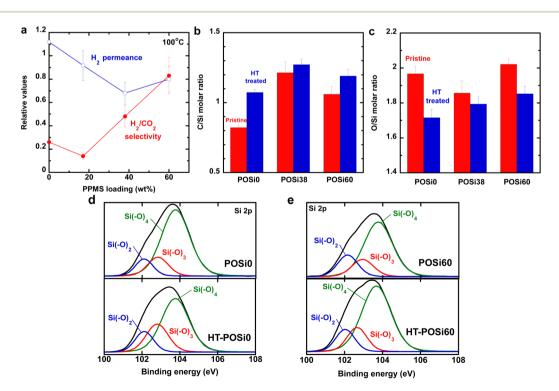
Fig. 5 Hydrothermal stability of POSi membranes after exposure to saturated water vapor at 100 °C for 12 h. (a) Relative H<sub>2</sub> permeance and H<sub>2</sub>/ CO<sub>2</sub> selectivity. (b) C/Si molar ratio and (c) O/Si molar ratio. Si 2p peak deconvolution of (d) POSiO and (e) POSiO.
