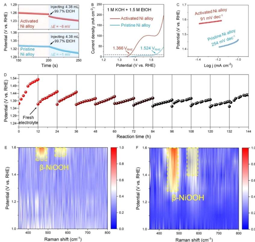
Fig. 4 (A) OCP test of pristine and activated Ni alloys before and after injecting EtOH. (B) LSV curves (with 90%  $iR$ -correction) of pristine and activated Ni alloys in 1 M KOH + 1.5 M EtOH at 5 mV s<sup>-1</sup>. (C) Corresponding Tafel plots. (D) Long-term stability. *In situ* Raman mapping plots of activated Ni alloys recorded in (E) 1 M KOH and (F) 1 M KOH + 1.5 M EtOH.
