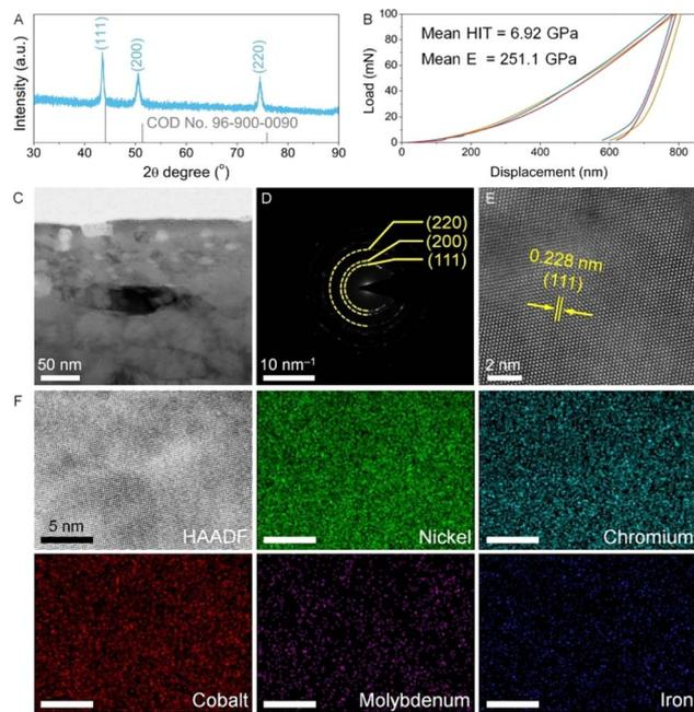
Fig. 1 (A) XRD pattern and (B) load–displacement curves of the as-prepared Ni alloy (HIT: indentation hardness;  $E$ : elastic modulus). TEM characterization of the Ni alloy: (C) TEM image, (D) SAED image, (E) high-resolution TEM image, (F) high-angle annular dark-field (HAADF) image and the corresponding elemental mapping.
