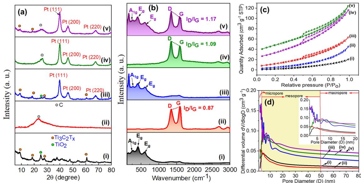
Fig. 2 (a) X-ray diffraction pattern, (b) Raman spectra, (c)  $N_2$  adsorption–desorption isotherms, and (d) pore size distribution curve of (i)  $Ti_3C_2T_x$ , (ii) rGO, (iii)  $Pt@Ti_3C_2T_x$ , (iv)  $Pt@rGO$  and (v)  $Pt@Ti_3C_2T_x-rGO$ .
