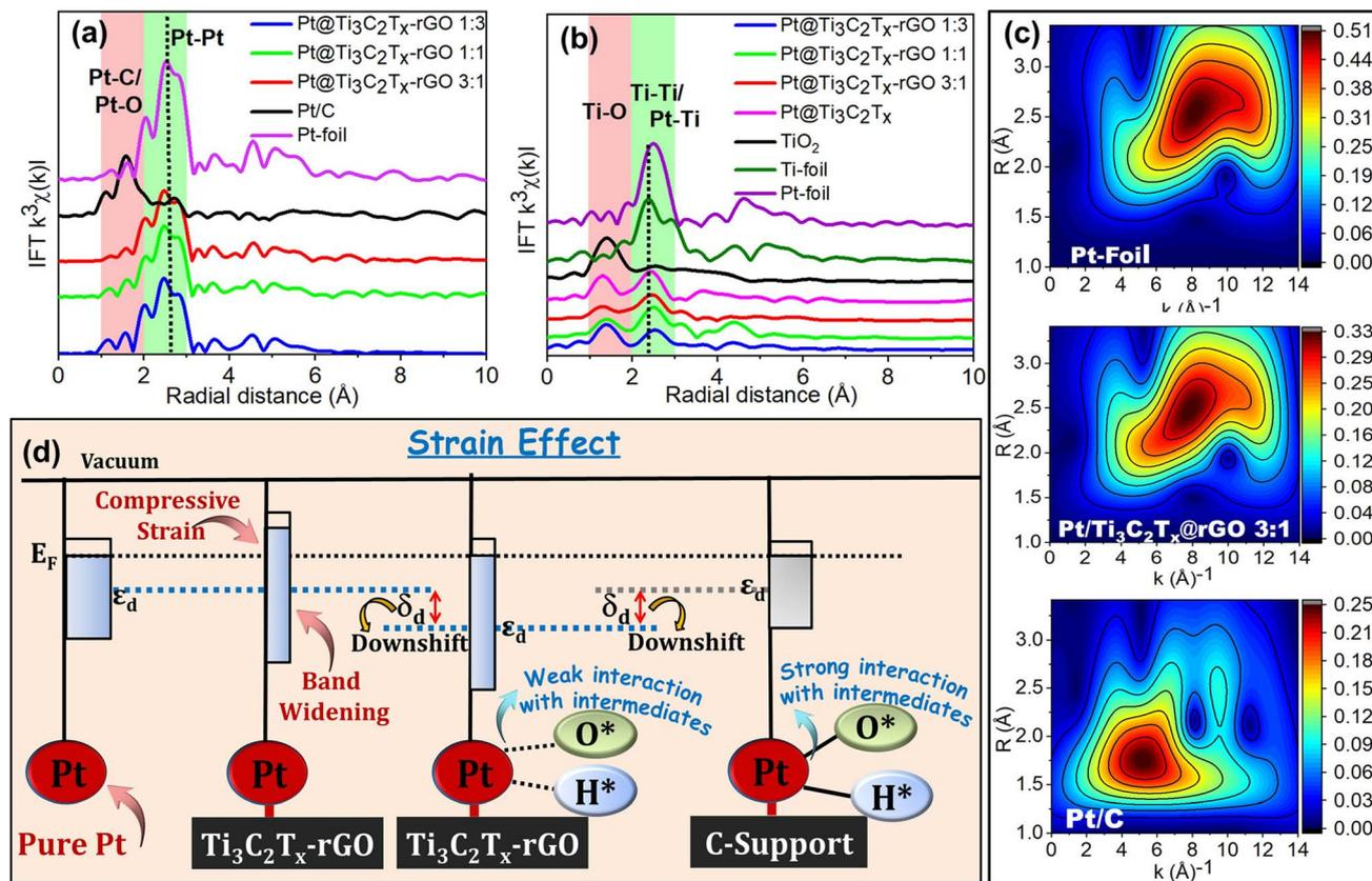
Fig. 8 Fourier transform-EXAFS (FT-EXAFS) oscillations of (a) the  $k^3$ -weighted Pt  $L_3$  edge and (b) the Ti K-edge. (c) Wavelet transforms (WT) of Pt@Ti<sub>3</sub>C<sub>2</sub>T<sub>x</sub>-rGO, Pt-foil and Pt/C for reference. (d) Schematic illustration of the effect of compressive strain on the bandwidth and the center of the d-band of Pt@Ti<sub>3</sub>C<sub>2</sub>T<sub>x</sub>-rGO with reference to Pt/C.
