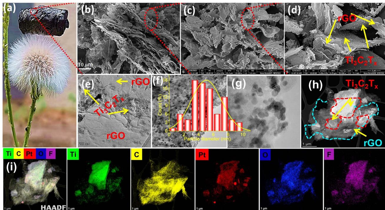
Fig. 3 (a) Photograph of the Pt@Ti<sub>3</sub>C<sub>2</sub>T<sub>x</sub>-rGO 3 : 1 aerogel placed on a dandelion, suggesting the featherweight density of the sample. (b)–(d) SEM images and (e)–(g) HR-TEM images (inset shows the particle size distribution histogram of Pt over Pt@Ti<sub>3</sub>C<sub>2</sub>T<sub>x</sub>-rGO 3 : 1) and (h)–(i) HAADF-STEM images and the corresponding elemental maps of Ti, C, Pt, O and F for Pt@Ti<sub>3</sub>C<sub>2</sub>T<sub>x</sub>-rGO 3 : 1.
