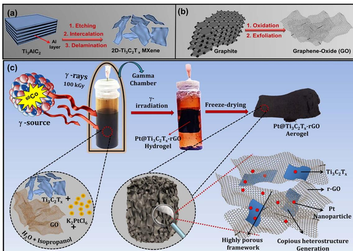
**Scheme 1** Graphical illustration outlining: (a) synthesis of 2D Ti<sub>3</sub>C<sub>2</sub>T<sub>x</sub> nanosheets from Ti<sub>3</sub>AlC<sub>2</sub> using wet etching method; (b) synthesis of GO nanosheets from natural graphite through a modified Hummers' process and (c) synthesis of 3D Pt@Ti<sub>3</sub>C<sub>2</sub>T<sub>x</sub>-rGO aerogel framework *via*  $\gamma$ -radiolysis process.
