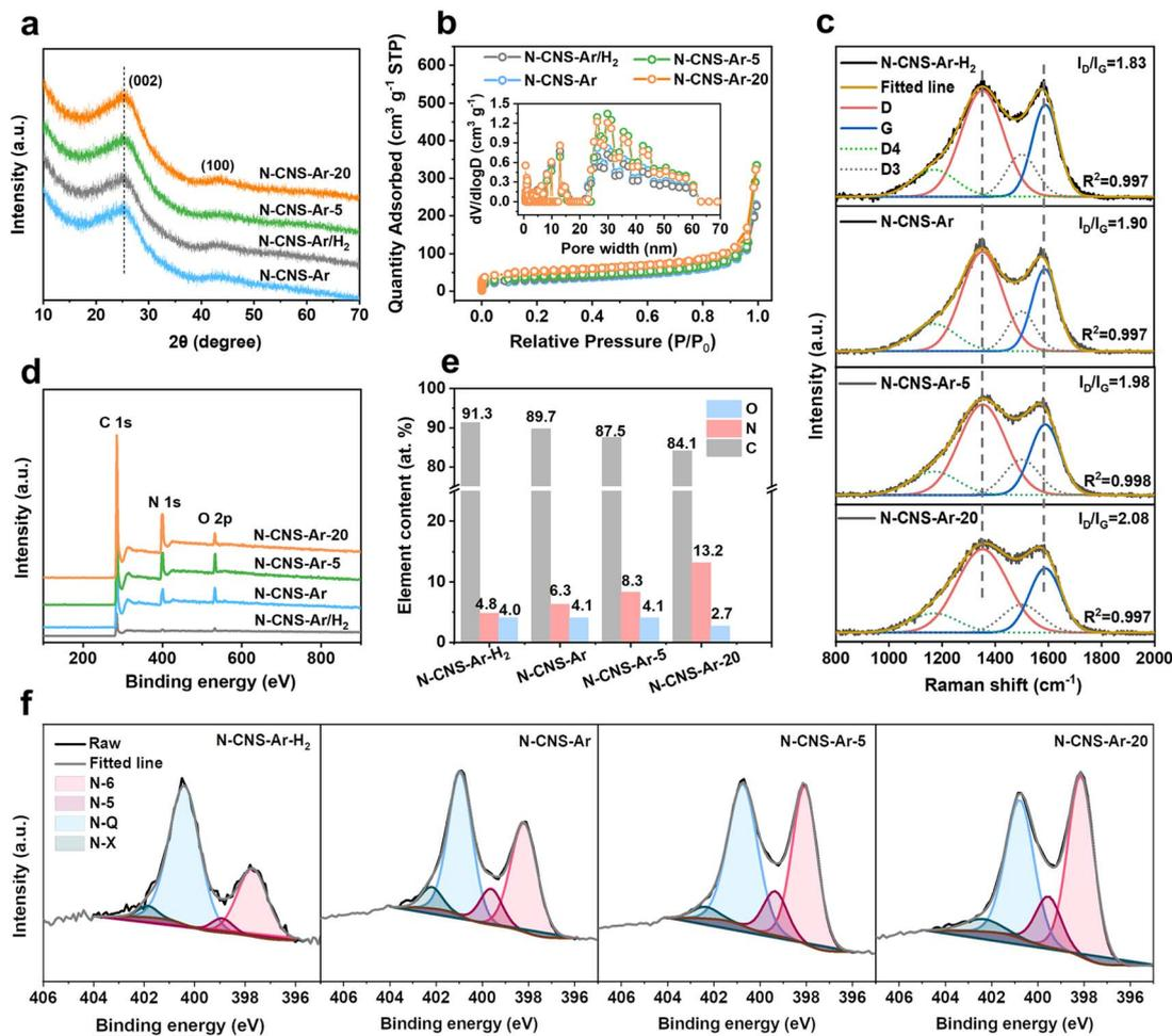
Fig. 2 Morphological and structural characterization of 2D crumpled N-CNS-Ar, N-CNS-Ar/H<sub>2</sub>, N-CNS-Ar-5, and N-CNS-Ar-20. (a) XRD patterns, (b) nitrogen adsorption–desorption isotherms (inset presents the pore size distributions obtained by the DFT method), (c) fitted Raman spectra curves, (d) XPS spectra, (e) element content of C, N and O, and (f) high-resolution N 1s XPS spectra.
