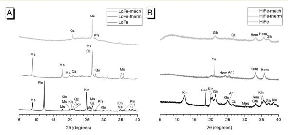
Fig. 1 XRD patterns for (A) LoFe as-received and activated clays, and (B) HiFe as-received and activated clays. Ant = anatase; Gbs = gibbsite; Gth = goethite; Hem = hematite; Kfs = K-feldspar; Kln = kaolinite; Mag = magnetite; Ms = muscovite; Qz = quartz. Plotted with normalised intensity (relative to the most intense peak in each pattern), for ease of readability.
