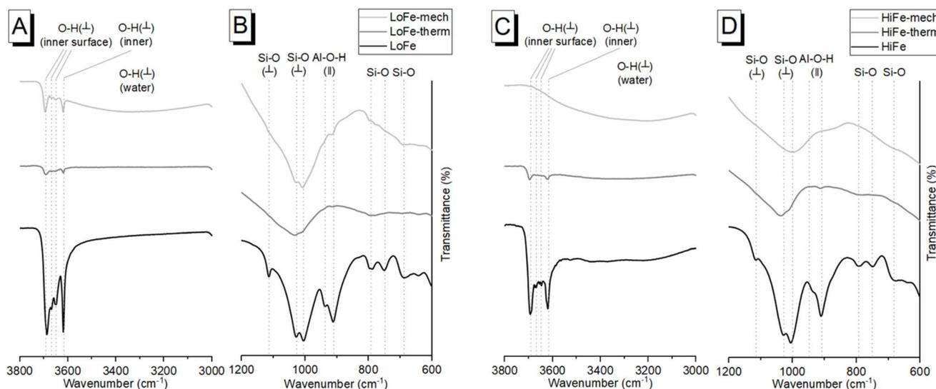
Fig. 3 For LoFe as-received and activated clays, FTIR spectra for (A) 3800–3000 cm<sup>-1</sup> and (B) 1200–600 cm<sup>-1</sup>. For HiFe as-received and activated clays, FTIR spectra for (C) 3800–3000 cm<sup>-1</sup> and (D) 1200–600 cm<sup>-1</sup>. ⊥ denotes a stretching vibration; || denotes a bending vibration.
