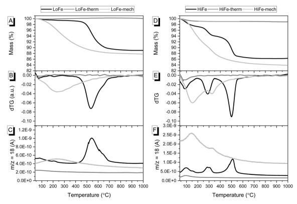
Fig. 2 For LoFe as-received and activated clays, curves for (A) TG, (B) dTG and (C) evolved H<sub>2</sub>O. For HiFe as-received and activated clays, curves for (D) TG, (E) dTG and (F) evolved H2O.
