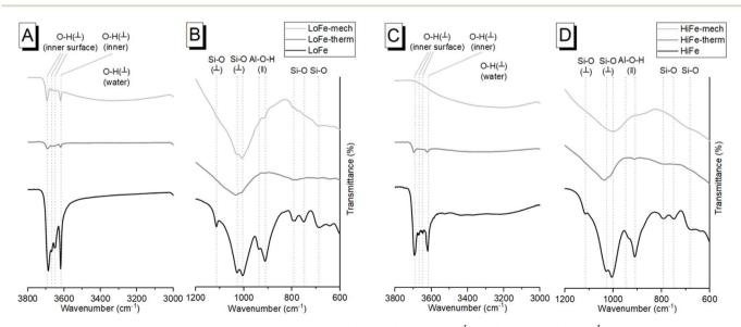
Fig. 3 For LoFe as-received and activated clays, FTIR spectra for (A) 3800–3000 cm<sup>-1</sup> and (B) 1200–600 cm<sup>-1</sup>. For HiFe as-received and activated clays, FTIR spectra for (C) 3800–3000 cm<sup>-1</sup> and (D) 1200–600 cm<sup>-1</sup>.  $\perp$  denotes a stretching vibration;  $\parallel$  denotes a bending vibration.
