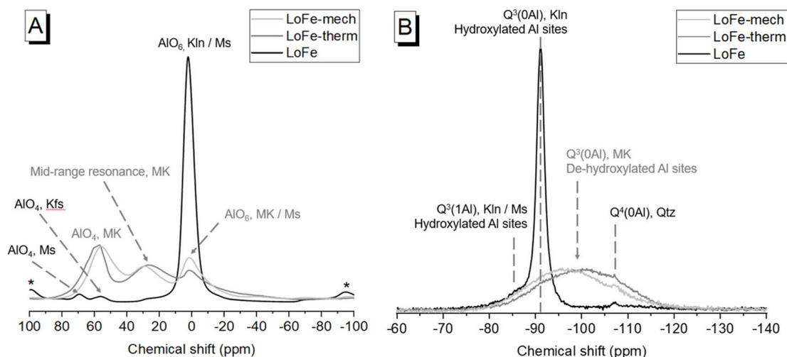
Fig. 7 A)  $^{27}\text{Al}$  MAS NMR spectra, and (B)  $^{29}\text{Si}$  MAS NMR spectra of the as-received LoFe, LoFe-therm and LoFe-mech clays. Mineral abbreviations are: Kln = kaolinite, Kfs = K-feldspar, MK = meta-kaolinite, Ms = muscovite, Qtz = quartz. \* symbols indicate the location of spinning side-bands.
