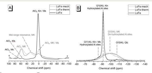
Fig. 7 A) <sup>27</sup>Al MAS NMR spectra, and (B) <sup>29</sup>Si MAS NMR spectra of the as-received LoFe, LoFe-therm and LoFe-mech clays. Mineral abbreviations are: KIn = kaolinite, Kfs = K-feldspar, MK = meta-kaolinite, Ms = muscovite, Qtz = quartz. \* symbols indicate the location of spinning side-bands.
