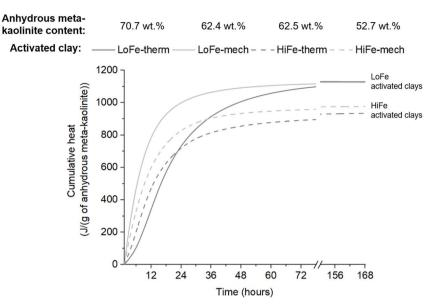
Fig. 11 A plot of cumulative heat curves, normalised to the estimated content of anhydrous meta-kaolinite in each activated clay. An x-axis break is used to show the closer convergence of the curves for each clay source by 168 hours.
