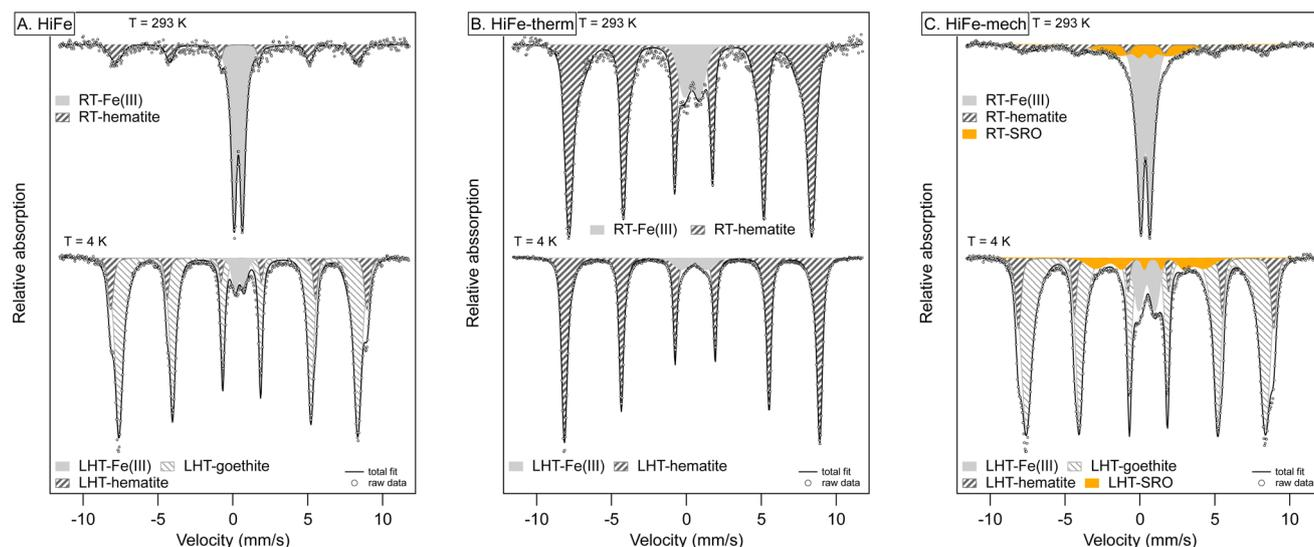
Fig. 9 Mössbauer spectra of HiFe clay as-received (A), after thermal treatment (B) and after mechanical treatment (C). Spectra were collected at room temperature (RT: 293 K) and at low temperature (LHT: 4 K). Hyperfine parameters of the Fe components used in the fit are listed in Table S5 in the ESI.†
