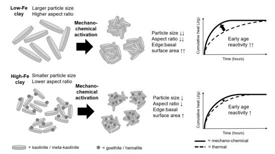
Fig. 12 Schematic showing the impact of the physical properties of the clays on chemical reactivity. A larger reduction in kaolinite primary particle size and aspect ratio for the mechano-chemically activated LoFe clay compared to the mechano-chemically HiFe clay can cause a higher relative increase in edge:basal surface area, leading to a greater increase in early age reactivity (in comparison to the thermal activation).
