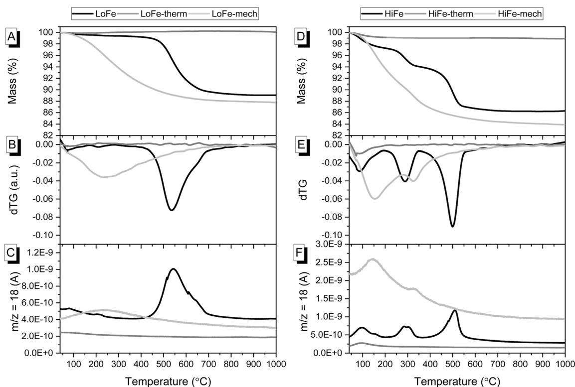
Fig. 2 For LoFe as-received and activated clays, curves for (A) TG, (B) dTG and (C) evolved  $\text{H}_2\text{O}$ . For HiFe as-received and activated clays, curves for (D) TG, (E) dTG and (F) evolved  $\text{H}_2\text{O}$ .
