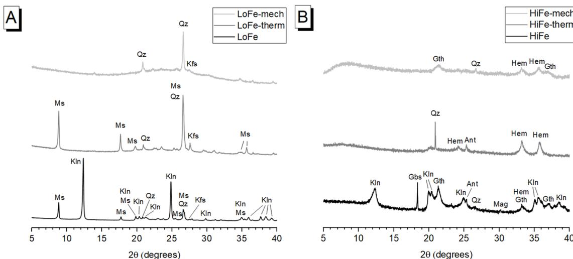
**Fig. 1** XRD patterns for (A) LoFe as-received and activated clays, and (B) HiFe as-received and activated clays. Ant = anatase; Gbs = gibbsite; Gth = goethite; Hem = hematite; Kfs = K-feldspar; Klin = kaolinite; Mag = magnetite; Ms = muscovite; Qz = quartz. Plotted with normalised intensity (relative to the most intense peak in each pattern), for ease of readability.
