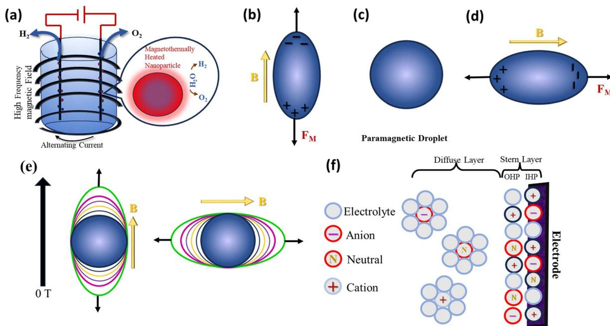
Fig. 7 (a) Localized heating of the magnetic nanoparticles on an electrode by an alternating magnetic field, leading to enhanced activity, (b–e) directional elongation of a paramagnetic droplet depending on the direction of the external magnetic field and (f) electrode/electrolyte interface, which is comprised a Stern and diffuse layer, where the former is sub-divided into the inner and outer Helmholtz planes.
