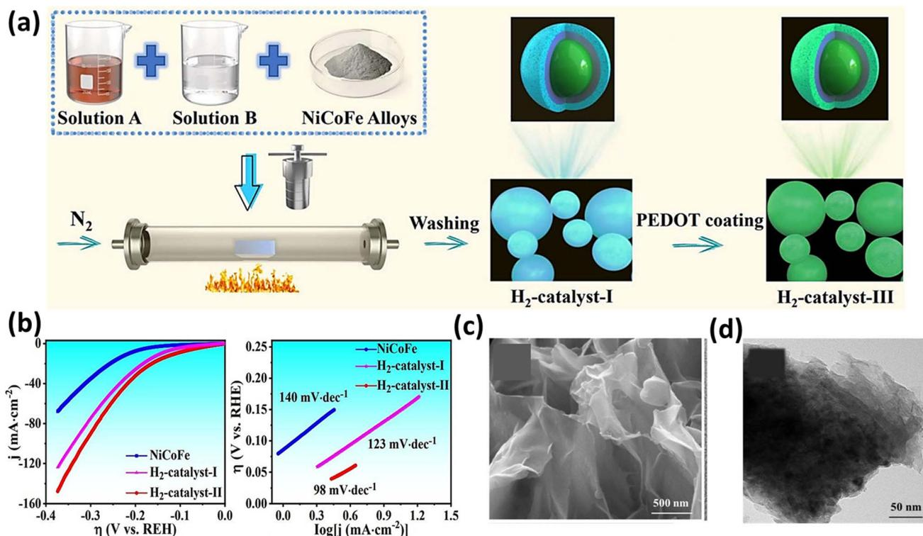
Fig. 13 (a) Schematic of the synthesis of NiCoFe electrocatalysts and (b) LSV and Tafel slope of the NiCoFe electrocatalysts (reprinted with permission,<sup>172</sup> copyright 2023, Elsevier). (c) and (d) SEM and HRTEM images of NiCo<sub>2</sub>S<sub>4</sub> (reprinted with permission,<sup>173</sup> copyright 2023, Elsevier).
