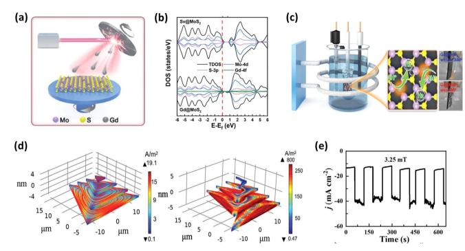
Fig. 15 (a) Schematic of laser molecular beam epitaxy to prepare Gd@MoS<sub>2</sub>, (b) DOS spectra of Gd@MoS<sub>2</sub> and Sv@MoS<sub>2</sub>, and (c) schematic of AMF-assisted electrochemical setup for HER analysis (reprinted with permission, 180 copyright 2022, Wiley). (d) Simulated Eddy current density of step and screw pyramid MoS<sub>2</sub> and (e) response of screw pyramid to AMF stimulation in HER (reprinted with permission, <sup>181</sup> copyright 2022, Wiley).
