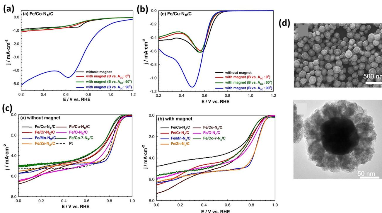
Fig. 22 (a) and (b) ORR polarization plots of Fe/Co-N<sub>x</sub>/C and Fe/Cu-N<sub>x</sub>/C, respectively, and (c) RRDE curves plotted in the presence and absence of a magnetic field for the above-mentioned electrocatalysts (reprinted with permission,<sup>215</sup> copyright 2022, Elsevier). (d) SEM and TEM images of Fe<sub>3</sub>O<sub>4</sub>-encapsulated Ag shells (reprinted with permission,<sup>214</sup> copyright 2020, the American Chemical Society).
