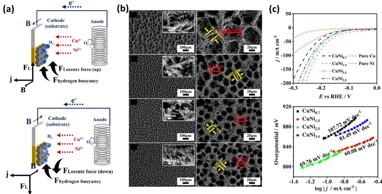
Fig. 10 (a) Schematic of magnetic field-controlled electrodeposition with upward and downward Lorentz force. (b) Low- and high-magnification images of CuNi films deposited with upward Lorentz force at different current densities. (c) LSV curves and Tafel plots of the electrocatalyst (reprinted with permission,<sup>157</sup> copyright 2024, Elsevier).
