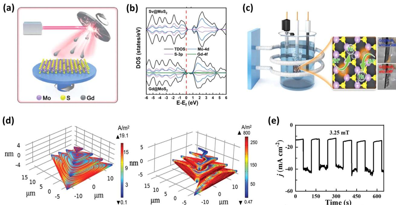
Fig. 15 (a) Schematic of laser molecular beam epitaxy to prepare Gd@MoS<sub>2</sub>, (b) DOS spectra of Gd@MoS<sub>2</sub> and Sv@MoS<sub>2</sub>, and (c) schematic of AMF-assisted electrochemical setup for HER analysis (reprinted with permission,<sup>180</sup> copyright 2022, Wiley). (d) Simulated Eddy current density of step and screw pyramid MoS<sub>2</sub> and (e) response of screw pyramid to AMF stimulation in HER (reprinted with permission,<sup>181</sup> copyright 2022, Wiley).
