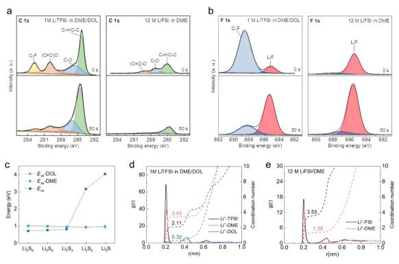
Fig. 3 High resolution (a) C 1s and (b) F 1s spectra of S cathodes cycled in 1 M LiTFSI in DME/DOL and 12 M LiFSI in DME at the etching times of 0 and 50 s. (c)  $E_{ce}$  of polysulfides and their  $E_{se}$  with DME and DOL. Coordination number distribution of (d) 1 M LiTFSI in DME/DOL and (e) 12 M LiFSI in DME.
