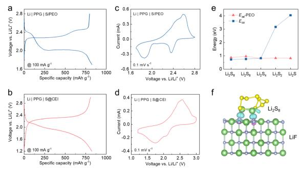
Fig. 4 (a and b) Galvanostatic voltage profiles and (c and d) CV curves at a scan rate of  $0.1 \,\mathrm{mV} \,\mathrm{s}^{-1}$  of (a and c) Li | PPG | S/PEO cell and (b and d) Li | PPG | S@CEI cell at 60 °C. (e)  $E_{ce}$  of polysulfides and their  $E_{se}$  with PEO. (f) Charge density difference between LiF and Li<sub>2</sub>S<sub>8</sub>. The light blue and purple sections represent the electron accumulation and loss parts, respectively.
