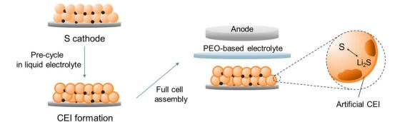
Schematic illustration of the artificial CEI formation on the S cathode and reassembly of the PEO-based all-solid-state Li-S battery.
