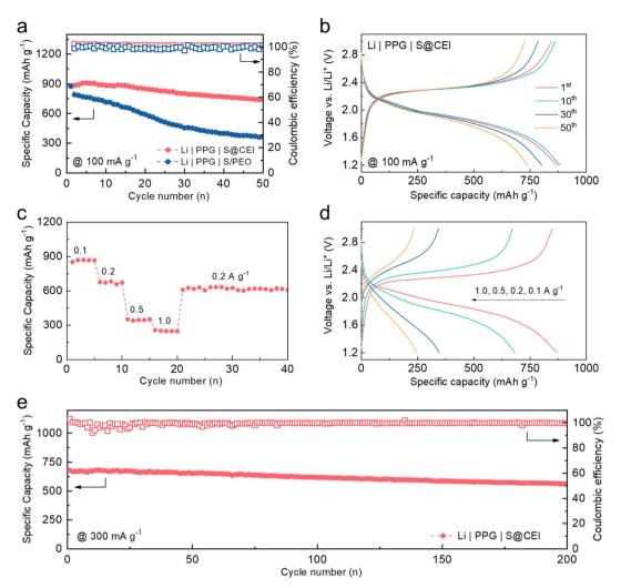
Fig. 5 (a) Discharge capacities of Li | PPG | S@CEI and Li | PPG | S/PEO cells at 100 mA g<sup>-1</sup> for 50 cycles. (b) Representative voltage profiles of the Li | PPG | S@CEI cell. (c) Discharge capacities and (d) voltage profiles of the Li | PPG | S@CEI cell at varying current densities. (e) Long-term cycling performance of the Li | PPG | S@CEI cell at 300 mA g<sup>-1</sup>. All cell tests were conducted at 60 °C
