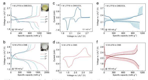
Fig. 2 (a and b) Galvanostatic voltage profiles ((insets): digital photos of separators retrieved from cycled cells), (c and d) CV curves at a scan rate of 0.1 mV s<sup>-1</sup>, and (e and f) GITT curves of Li-S cells using (a, c and e) 1 M LiTFSI in DME/DOL and (b, d and f) 12 M LiFSI in DME.
