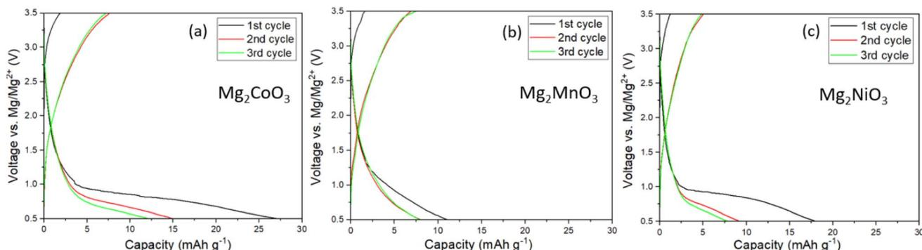
Fig. 3 Electrochemistry of Mg-rich disordered rocksalts. Charge/discharge profiles of the first three cycles of (a)  $\text{Mg}_2\text{CoO}_3$ , (b)  $\text{Mg}_2\text{MnO}_3$ , and (c)  $\text{Mg}_2\text{NiO}_3$  in Mg cells at 60 °C using 0.3 M  $\text{Mg}[\text{B}(\text{hfp})_4]_2$  in DME as the electrolyte at a current density of 10  $\text{mA g}^{-1}$ .
