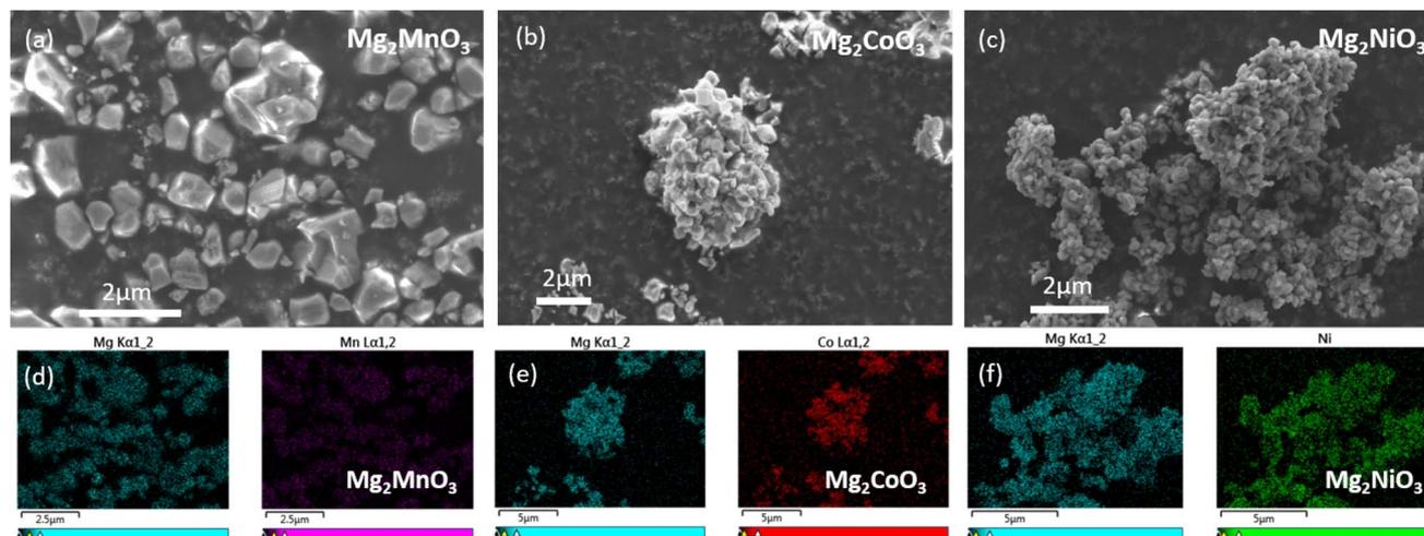
Fig. 2 Particle morphology and uniform elemental distribution. SEM and EDX of the  $\text{Mg}_2\text{TMO}_3$  samples. SEM images of (a)  $\text{Mg}_2\text{MnO}_3$ , (b)  $\text{Mg}_2\text{CoO}_3$ , and (c)  $\text{Mg}_2\text{NiO}_3$  showing primary particle sizes from 0.1 to 1  $\mu\text{m}$ . EDX elemental mapping of (d)  $\text{Mg}_2\text{MnO}_3$ , (e)  $\text{Mg}_2\text{CoO}_3$ , and (f)  $\text{Mg}_2\text{NiO}_3$ , which shows homogeneous distribution of elements in the samples.
