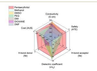
Fig. 1 Radar map screening seven different electrolyte additives for aqueous ZIBs by considering cost, conductivity, safety H-bond donor/acceptor number and dielectric coefficient.
