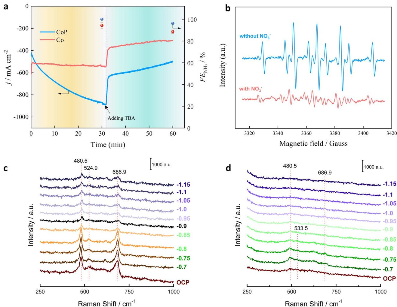
Fig. 4 (a)  $j$  and  $\text{FE}_{\text{NH}_3}$  over Co-P@NF and Co@NF at potential of  $-0.1 \text{ V}$  vs. RHE. (b) The DMPO-H\* obtained on Co-P@NF after 5 min of electrocatalysis at  $-0.1 \text{ V}$  vs. RHE in  $1 \text{ M KOH}$  solution with  $0.1 \text{ M NO}_3^-$  (bottom) or (b) without  $\text{NO}_3^-$  (top). *In situ* electrochemical-Raman on Co-P (c) and Co (d) in the potential of  $-0.7 \text{ V}$ – $-1.15 \text{ V}$  vs. Hg/HgO.
