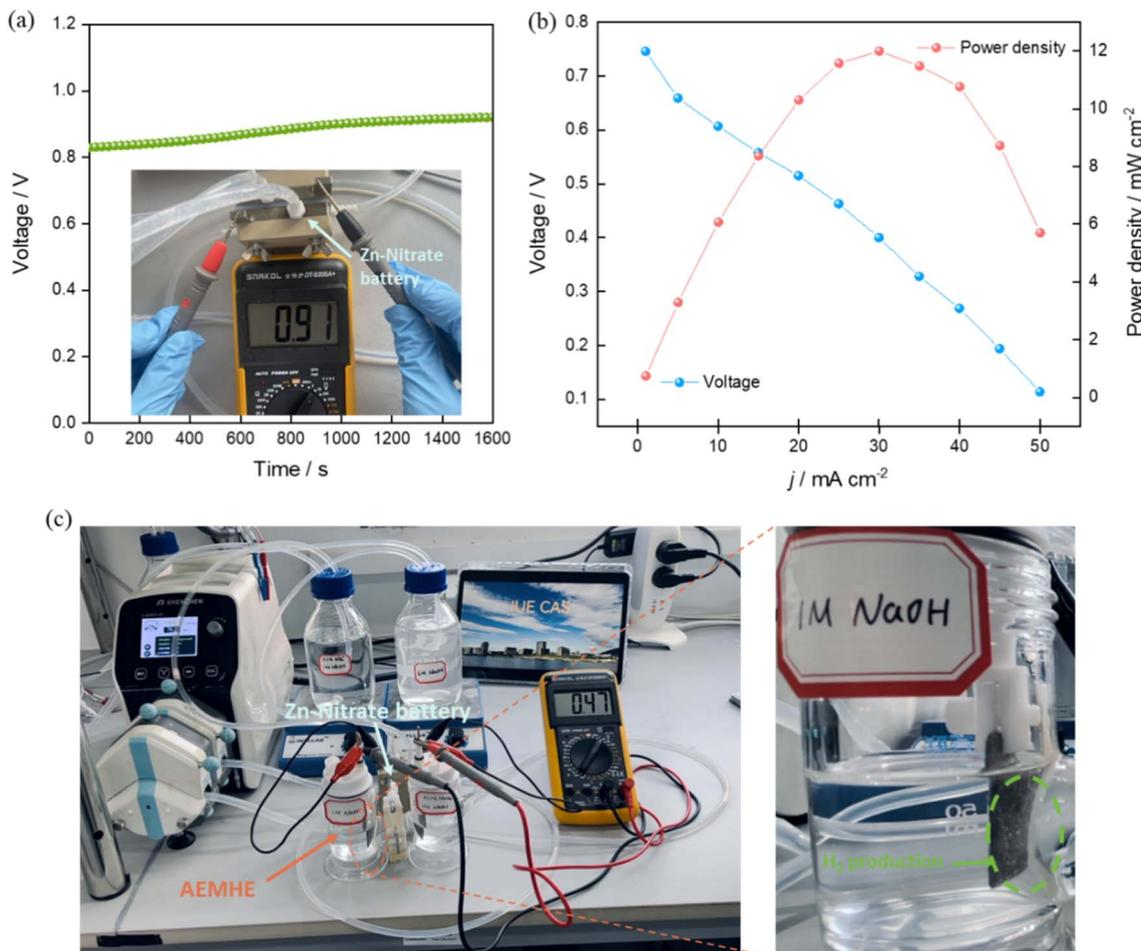
Fig. 6 Zn-nitrate flow battery application. (a) The open circuit voltage. The cathodic and anodic electrolytes used in Zn-nitrate flow battery were 0.1 M  $\text{NO}_3^-$  + 1 M NaOH and 6 M NaOH, respectively. (b) Polarization and power density curves. (c) The digital photograph of the tandem Zn-nitrate flow battery and AEMHE devices for hydrogen production.
