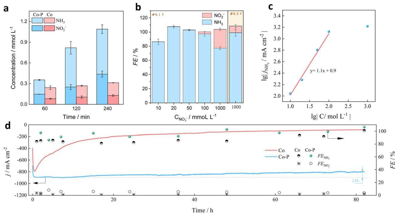
Fig. 3 (a) Concentration of  $\text{NO}_2^-$  and  $\text{NH}_3$  over Co-P@NF and Co@NF at open circle potential. (b) FE of  $\text{NO}_2^-$  and  $\text{NH}_3$  and (c)  $\lg(-j)$  vs.  $\lg C$  plots for Co-P@NF were calculated at  $-0.1 \text{ V}$  vs. RHE. (d) Long-term stability of Co-P@NF in the electrolyte of  $1 \text{ mol L}^{-1}$  with  $100 \text{ mmol L}^{-1}$   $\text{NO}_3^-$  at  $-0.1 \text{ V}$ .
