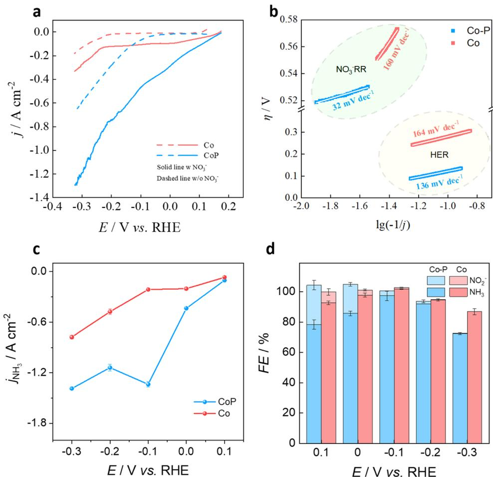
Fig. 2 (a) Linear sweeping voltammetry over Co@NF and Co-P@NF in the electrolyte of 1 mol L<sup>-1</sup> KOH with or without 100 mmol L<sup>-1</sup> NO<sub>3</sub><sup>-</sup>. (b) Tafel slope of Co@NF and Co-P@NF in the presence of NO<sub>3</sub><sup>-</sup>. (c) Partial current density of NH<sub>3</sub> production over Co@NF and Co-P@NF. (d) FE of NH<sub>3</sub> and NO<sub>2</sub><sup>-</sup> over Co-P@NF and Co@NF in the potential range of 0.1–-0.3 V.
