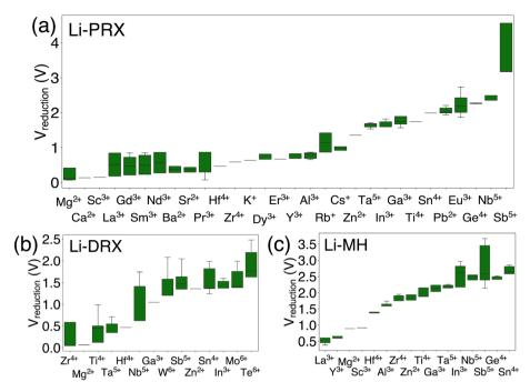
Fig. 1 The metal dependent reduction voltage (referenced to Li/Li<sup>+</sup>) of (a) Li perovskite (Li-PRX), (b) Li disordered rocksalt (Li-DRX) and (c) Li metal halide (Li-MH) compounds.
