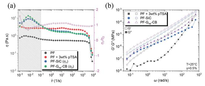
Fig. 2 Rheological studies showing (a) the change in viscosity with the addition of acid catalyst (pTSA) and dispersions of SiC and  $G_{np}$ -CB nanoparticles. The pink stars indicate the viscosity ratio around 1 between PF-SiC and PF- $G_{np}$ -CB and (b) flow sweep highlighting the storage and loss moduli of the feedstocks.
