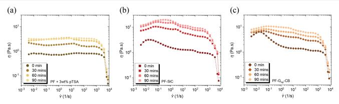
Fig. 3 Flow sweep indicating the change in viscosity with the addition of pTSA as a function of time at the room temperature (RT) for as-prepared feedstocks (a) PF resin, (b) PF-SiC, and (c) PF- $G_{np}$ -CB.
