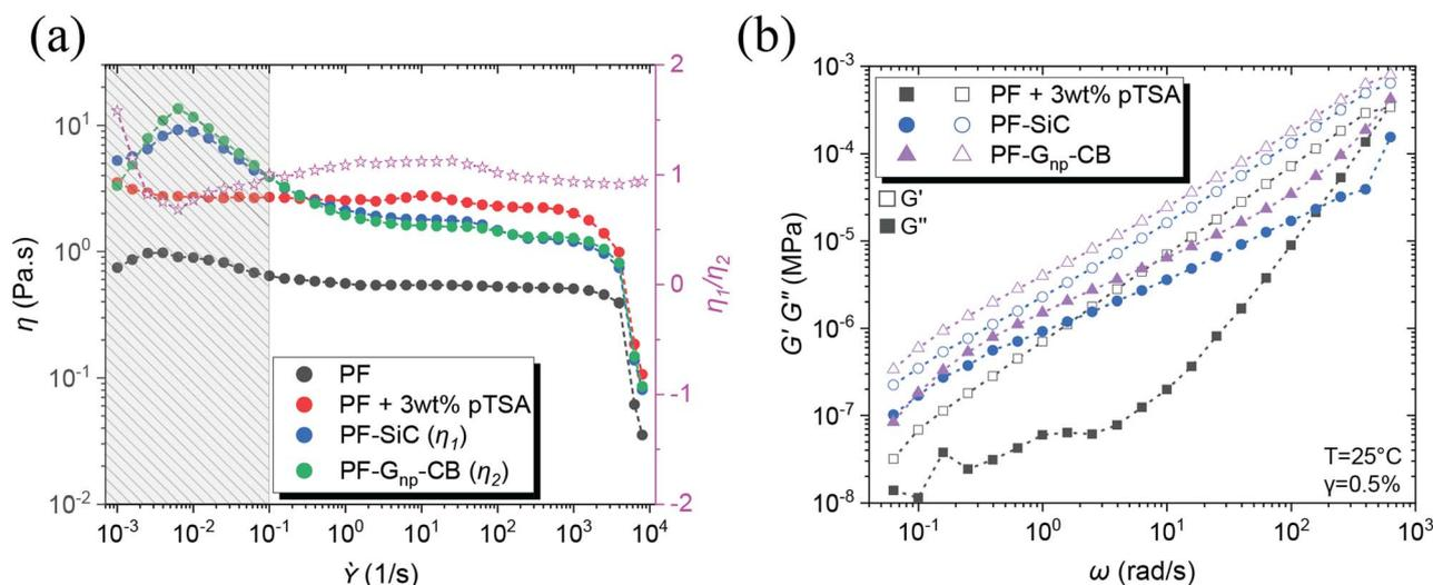
Fig. 2 Rheological studies showing (a) the change in viscosity with the addition of acid catalyst (pTSA) and dispersions of SiC and  $G_{np}$ -CB nanoparticles. The pink stars indicate the viscosity ratio around 1 between PF-SiC and PF- $G_{np}$ -CB and (b) flow sweep highlighting the storage and loss moduli of the feedstocks.
