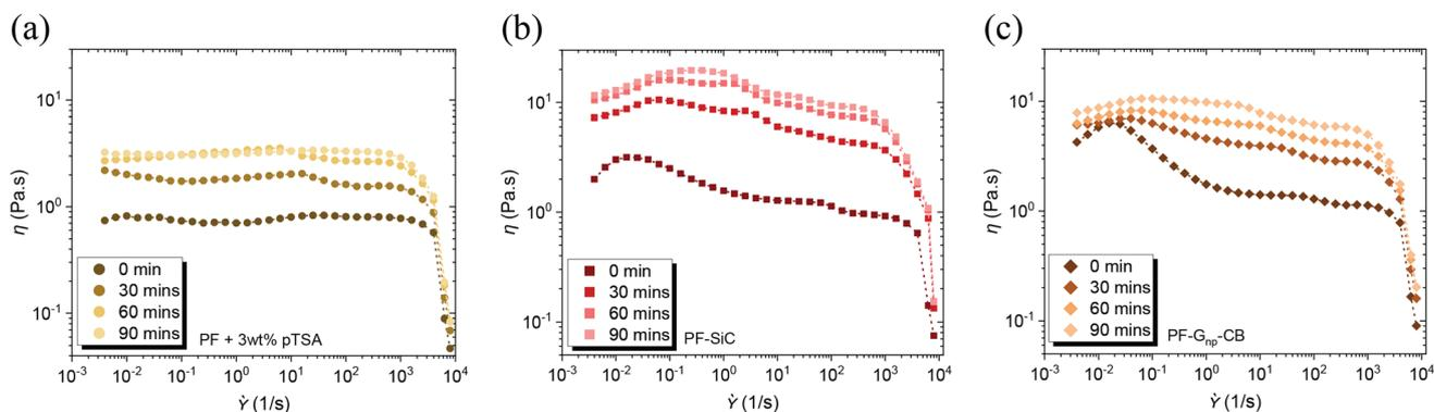
Fig. 3 Flow sweep indicating the change in viscosity with the addition of pTSA as a function of time at the room temperature (RT) for as-prepared feedstocks (a) PF resin, (b) PF-SiC, and (c) PF-G<sub>np</sub>-CB.
