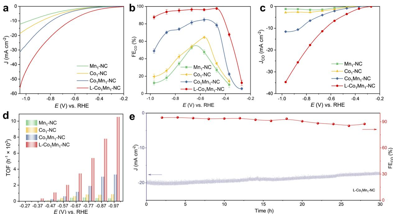
Fig. 3 The CO<sub>2</sub>RR performance of L-Co<sub>1</sub>Mn<sub>1</sub>-NC, Co<sub>1</sub>Mn<sub>1</sub>-NC, Co<sub>1</sub>-NC, and Mn<sub>1</sub>-NC catalysts. (a) LSV profiles. (b) FE<sub>CO</sub> curves. The error bars correspond to the standard deviation of three independent measurements. (c) *J*<sub>CO</sub> curves. (d) TOF comparison image. (e) The stability test curve of the L-Co<sub>1</sub>Mn<sub>1</sub>-NC catalyst at –0.8 V.
