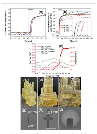
Fig. 1 Photo-rheology (a) complex viscosity and (b) dynamic time sweep curves (storage (solid) and loss (dashed) modulus vs. time), with varying ARO/IBOA ratios at 22 °C. (c) DSC first and second heating scan of 3D printed samples and the rheology temperature ramp curve for uncured resin. Images of a 3D printed (d) castle model with (e and f) close-up photos and SEM images of an in-cut of (g) 0.2 mm and (h) 0.5 mm and (i) a dome demonstrating separate layer lines
