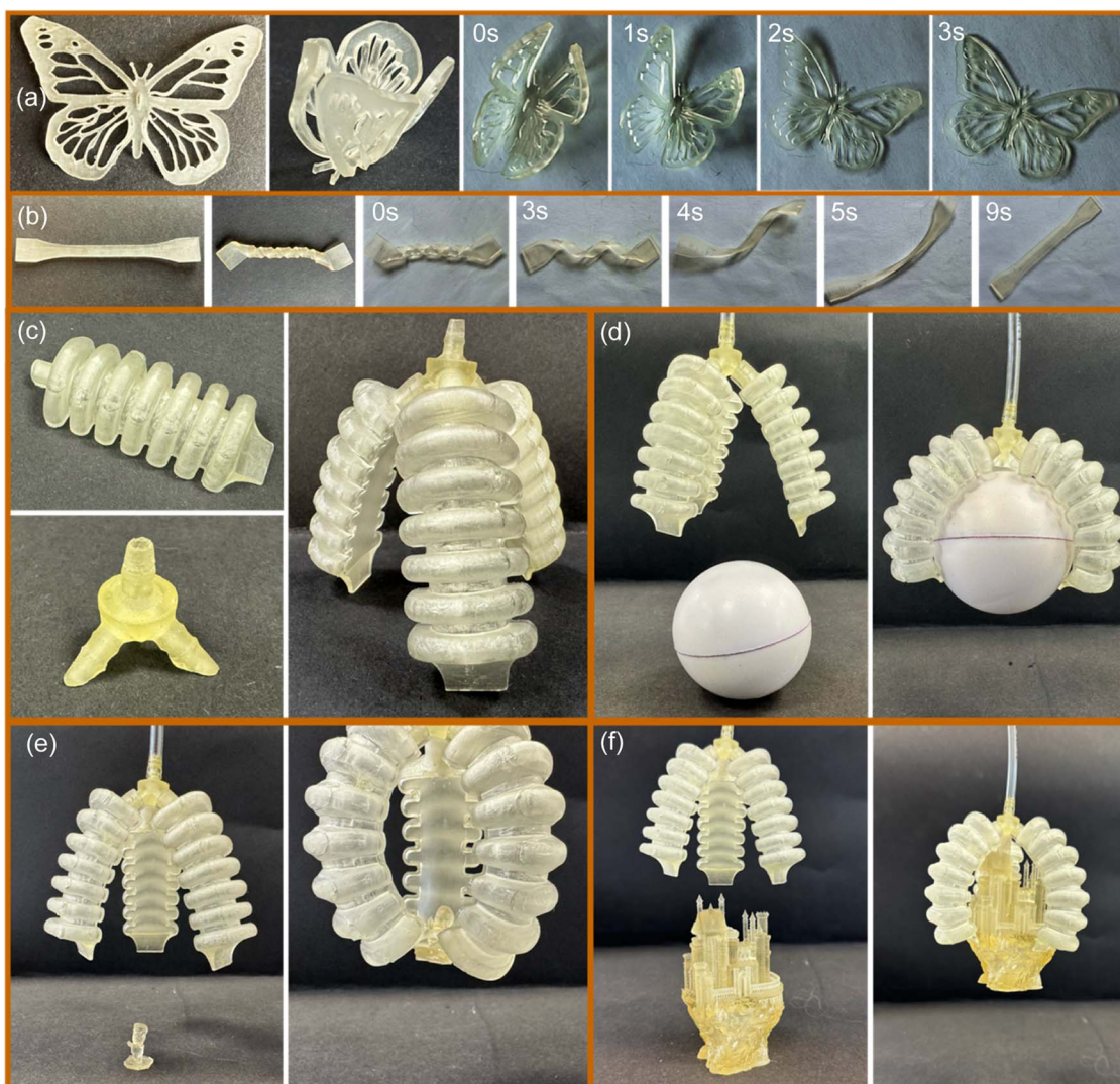
Fig. 7 Images of shape memory demonstration of the 3D printed (a) butterfly model, (b) dog-bone shaped sample, (c) tri-Y splitter, and assembled soft robotic gripper holding a (d) ball, (e) small 3D printed figure of irregular shape, and (f) large 3D printed object of irregular shape.
