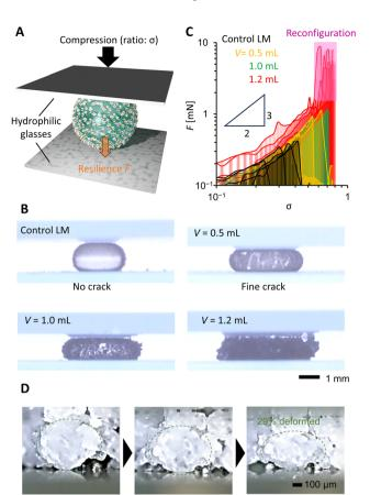
Fig. 4 (A) Scheme of the compression test. (B) Side view of the compressed PGLM just before breakage with 10  $\mu L$  water. (C) Compression–resilience curve of the PGLM with 10  $\mu L$  water in different PDMS volumes. Resilience fluctuation region (pink highlighted) is owing to the PG reconfiguration. (D) Side-view microscopic image monitoring the deformation of the PG (V = 1.2 mL) during the deformation of the PGLM by a glass plate. The observed PG deformed by around 29% in height.
