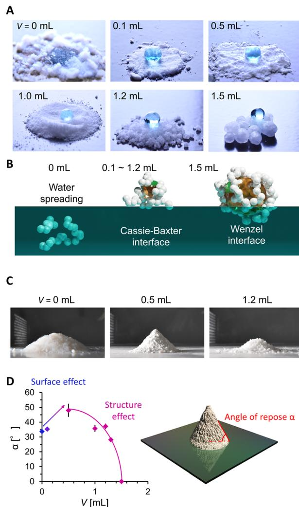
Fig. 3 (A) 20  $\mu\text{L}$  water droplets on PG. (B) Water adhesion states on PG estimated from water contact behaviors. (C) Shape of particles or the PG powder mountain. (D) Angle of repose evolution.
