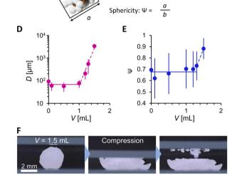
Fig. 2 (A) PDMS volume effect on PG. (B) Digital microscopic images. (C) Scheme explaining PG geometry analysis. (D) Diameter and (E) sphericity of PG. (F) Mechanical shape reconfiguration of PG.
