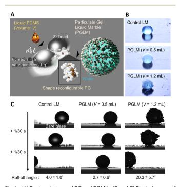
Fig. 1 (A) Design strategy of PG and PGLMs. (B and C) Photo images of a classical LM and a PGLM (B) resting and (C) rolling-off on the tilted glass substrate. Water volume is constant at 10  $\mu$ L. Rolling-off angle tends to increase with the roughness of the PGLM.
