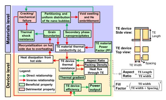
Fig. 6 Relationship map of factors to consider for TE device design in fusion reactors.
