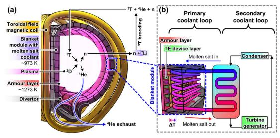
Fig. 1 (a) Cross-section schematic of a tokamak reactor running on the D-T fusion reaction. (b) Molten salt coolant loop inside each blanket module and a potential application of a TE device to harvest the thermal gradient between the armour layer and the molten salt coolant.
