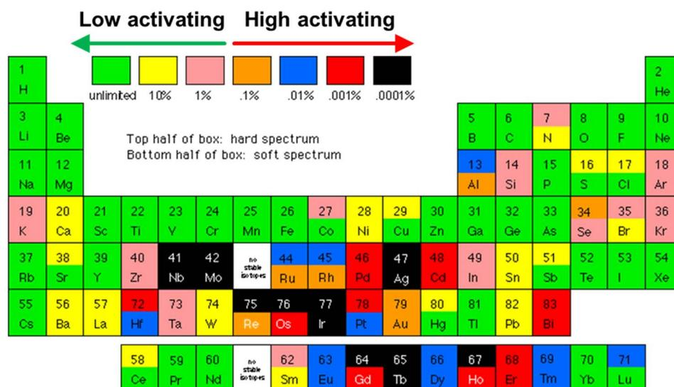
Fig. 4 Periodic table of low and high activation elements, assuming a 5 MW m<sup>-2</sup> flux for 4 years. Image obtained from the open web [http://qedfusion.org/LIB/PROPS/SAFETY/class\_c.shtml] on 29 Mar 2024.
