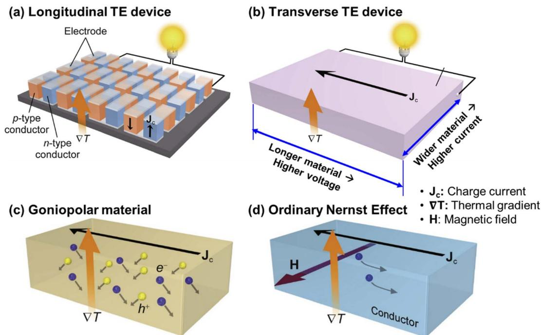
Fig. 7 Schematic diagrams of (a) a traditional longitudinal TE device, (b) a transverse TE device, and transverse TE transport (c) using a goniopolar material and (d) using the ordinary Nernst effect. Copyright 2022, Elsevier Inc. Adapted with permission from ref. 152, Elsevier Inc.
