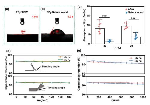
Fig. 5 The intrinsic flexibility of the AF-FSC at 20 or -30 °C. Contact angle of (a) PPy/ADW, (b) PPy/natural balsa wood after dropping a water droplet for 1.0 s at 20 °C. (c) Corresponding electrolyte absorption ability of PPy/ADW (red bar) and natural balsa wood (blue bar) at 20 and -30 °C. Capacitance retention of AF-FSC (d) under different bending/twisting angles; (e) after 1000 bending/twisting cycles.
