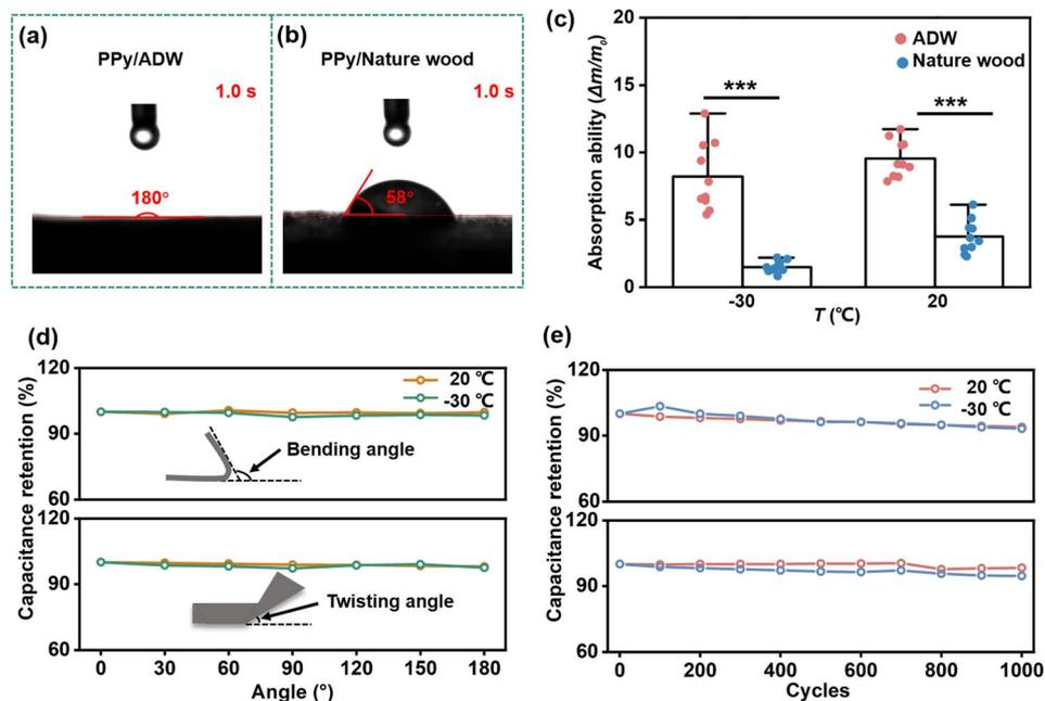
Fig. 5 The intrinsic flexibility of the AF-FSC at 20 or  $-30$  °C. Contact angle of (a) PPY/ADW, (b) PPY/natural balsa wood after dropping a water droplet for 1.0 s at 20 °C. (c) Corresponding electrolyte absorption ability of PPY/ADW (red bar) and natural balsa wood (blue bar) at 20 and  $-30$  °C. Capacitance retention of AF-FSC (d) under different bending/twisting angles; (e) after 1000 bending/twisting cycles.
