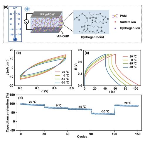
Fig. 4 The anti-freezing property of the SC. (a) Schematic illustration of the SC at -30 °C. Comparison of (b) CV and (c) GCD curves of the SC at temperatures of 20, 0, -15 and -30 °C. (d) Cycling performance of the SC at 20, 0, -15 and -30 °C. Scan rate of CV: 100 mV s<sup>-1</sup>; current density of GCD: 6 mA cm<sup>-2</sup>
