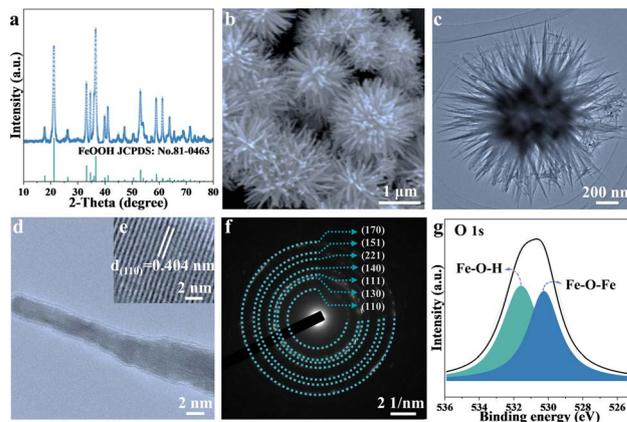
Fig. 1 Structural characterization of  $\text{FeOOH}$  anodes. (a) XRD pattern. (b) SEM image. (c) TEM image. (d) HRTEM image of the nanorod and (e) lattice fringe inside. (f) SAED image. (g) The high resolution XPS of O 1s.
