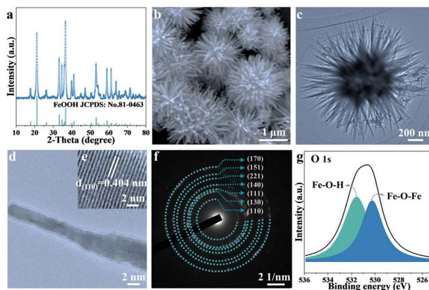
Fig. 1 Structural characterization of FeOOH anodes. (a) XRD pattern. (b) SEM image. (c) TEM image. (d) HRTEM image of the nanorod and (e) lattice fringe inside. (f) SAED image. (g) The high resolution XPS of O 1s.
