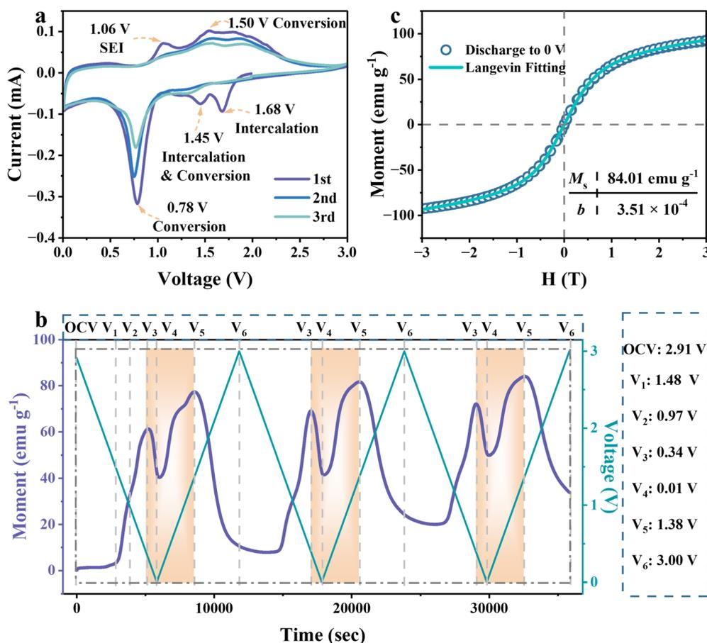
Fig. 2 Electrochemical reaction mechanism of FeOOH LIBs. (a) CV curves for the first three cycles at a scan rate of 0.5 mV s<sup>-1</sup> over the voltage range of 0.01–3 V. (b) Operando magnetic monitoring followed the voltage range of CV scanning under a magnetic field of 3 T. (c) Magnetic hysteresis loop with the Langevin fitting curve after the first full discharge measured at 300 K.
