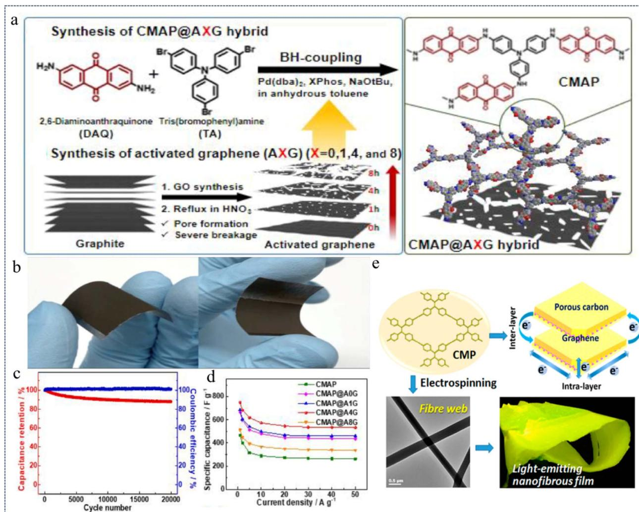
Fig. 24 (a) Synthesis of the CMAP@AXG hybrid. (b) Photographs of flexible CMAP@A4G electrodes. (c) Specific capacitance obtained at different scan rates from 1 to 50 A g<sup>-1</sup>. (d) Capacitance retention and coulombic efficiency test charts at a current density of 10 A g<sup>-1</sup>.<sup>147</sup> Copyright 2022, Elsevier. (e) Schematic diagram of electron transfer in graphene templated CMPs.<sup>41</sup> Copyright 2015, American Chemical Society.
