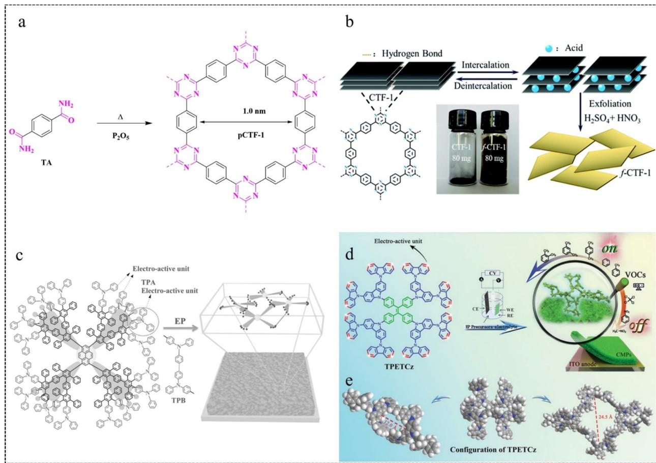
Fig. 8 (a) Synthesis of pCTF-1.<sup>75</sup> Copyright 2018, Wiley. (b) Preparation process of f-CTF-1 nanosheets.<sup>76</sup> Copyright 2019, Royal Society of Chemistry. (c) Dimerisation of TPA with TPB and schematic representation of the crosslinked network microstructure of EP membranes.<sup>80</sup> Copyright 2016, Wiley. (d) EP preparation of TPETCz-CMP films. (e) Structural model of TPETCz-CMP.<sup>26</sup> Copyright 2020, Wiley.
