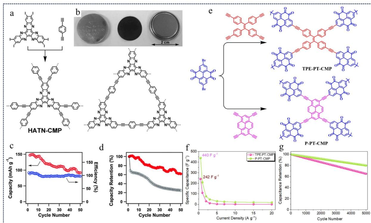
Fig. 2 (a) Synthesis of HATN-CMP networks. (b) The photos of HATN-CMP electrodes. (c) Cycle stability and (d) capacity retention ratio of HATN-CMP.<sup>44</sup> Copyright 2014, Royal Society of Chemistry. (e) Synthetic pathway of TPE-PT-CMP and P-PT-CMP. (f) Capacitance retention and (g) Ragone curve.<sup>45</sup> Copyright 2022, American Chemical Society.
