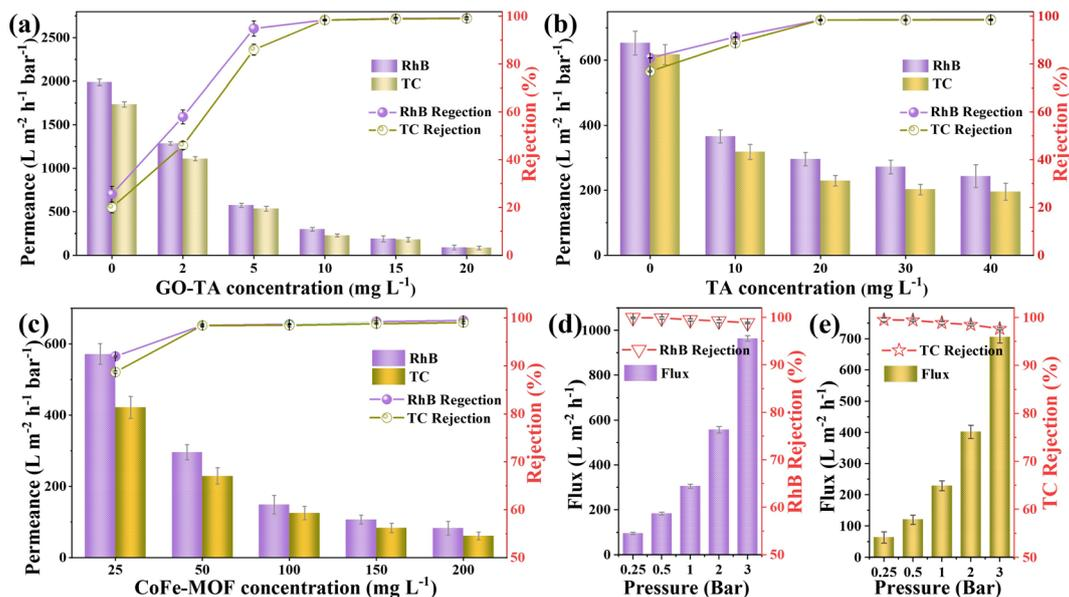
Fig. 4 Effects of GO-TA concentration (a), TA concentrations (b), CoFe-MOF concentration (c), and operating pressure (d and e) on separation performance.
