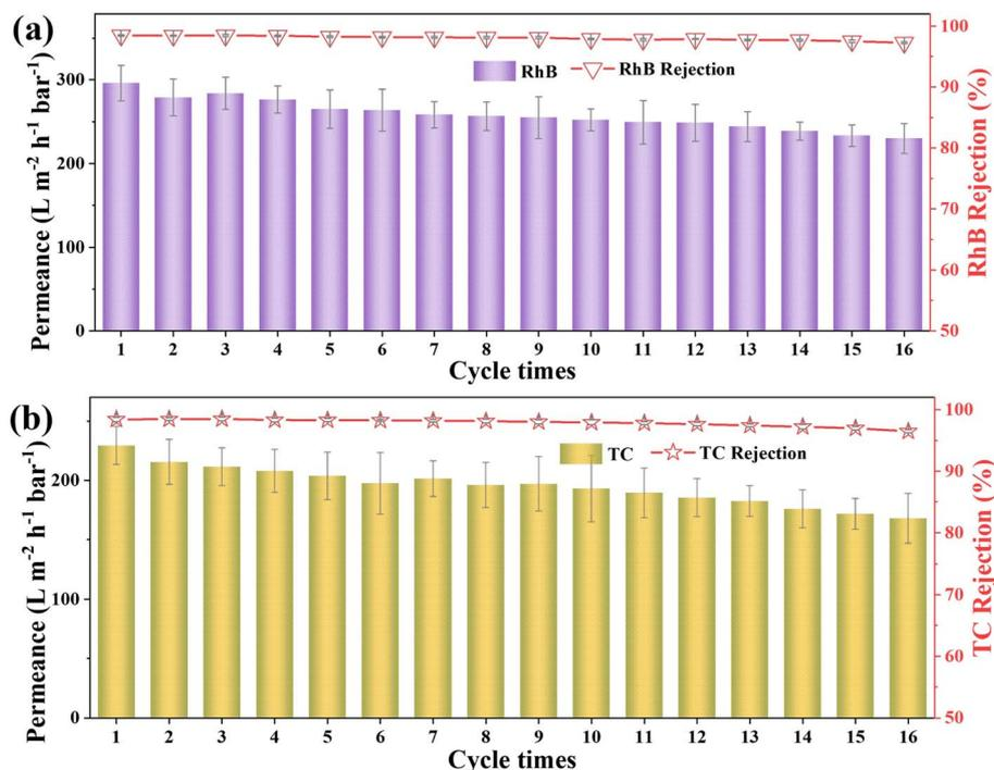
Fig. 8 Cycling separation performance of CoFe-MOF/GO-TA-10 for RhB (a) and TC (b). Conditions: [P] = 1.0 bar, [RhB] = 10 mg L<sup>-1</sup>, [PMS] = 100 mg L<sup>-1</sup>.
