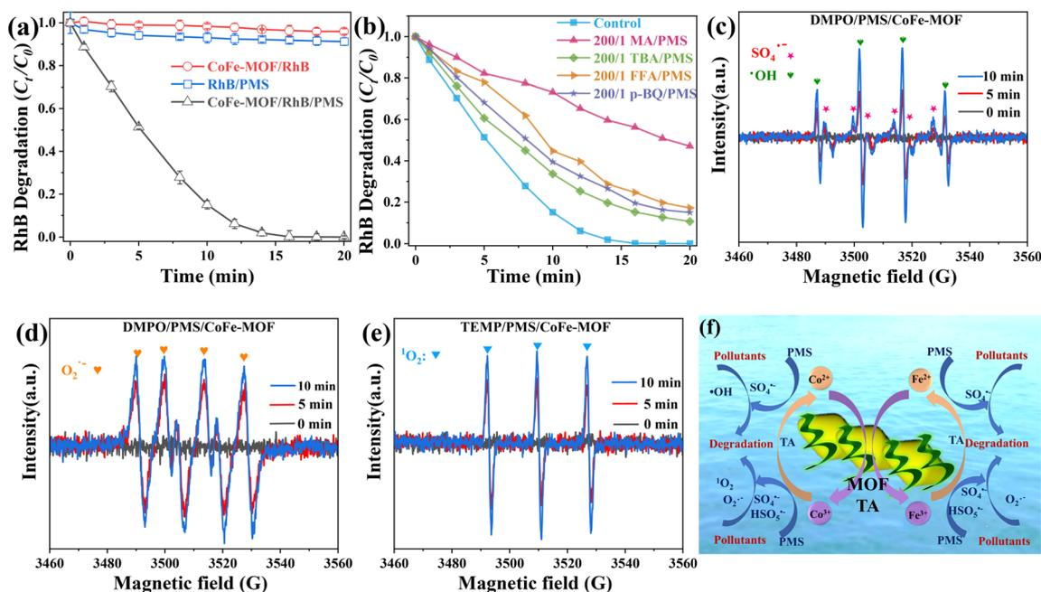
Fig. 6 Degradation process (a) and radical quenchers (b) in the CoFe-MOF/PMS/RhB system, EPR spectra of DMPO- $\text{HO}\cdot$  and DMPO- $\text{SO}_4^{\cdot-}$  (c), DMPO- $\text{O}_2^{\cdot-}$  (d) and TEMP- $^1\text{O}_2$  (e) and the degradation mechanism (f) in the CoFe-MOF/PMS system. Conditions: [catalyst] = 20 mg L<sup>-1</sup>, [RhB] = 20 mg L<sup>-1</sup>, [PMS] = 100 mg L<sup>-1</sup>.
