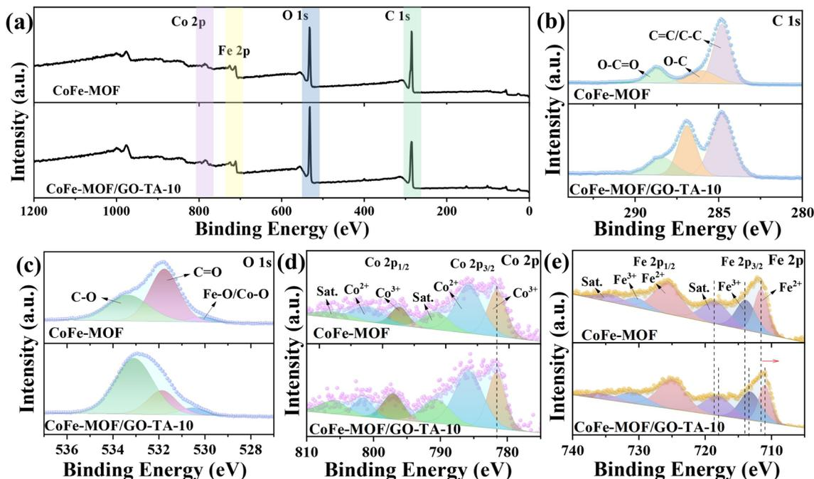
Fig. 3 XPS survey spectra (a), C 1s (b), O 1s (c), Co 2p (d), and Fe 2p (e) XPS spectra of CoFe-MOF and CoFe-MOF/GO-TA-10.
