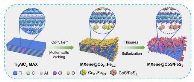
Fig. 1 Illustration for the synthesis of MXene@CoS/FeS2.
