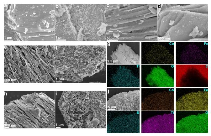
Fig. 2 SEM images of (a)  $Ti_3AlC_2$  MAX, (b) MAXNaCl/KCl, (c, d) MAX@NaCl/KCl–S, (e, f) MXene@Co<sub>0.7</sub>Fe<sub>0.3</sub>, and (h, i) MXene@CoS/FeS<sub>2</sub>. (g) EDS elemental mapping images of (g) MXene@Co<sub>0.7</sub>Fe<sub>0.3</sub> and (j) MXene@CoS/FeS<sub>2</sub>.
