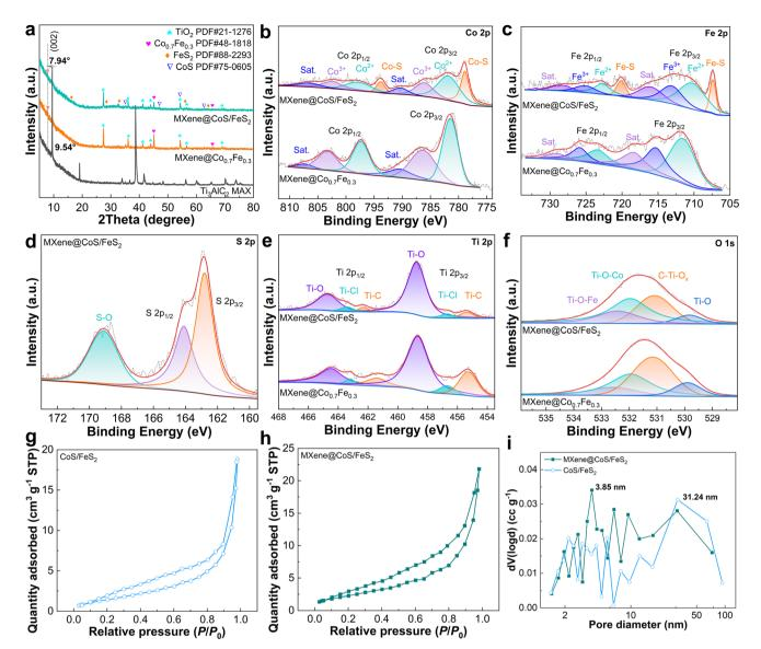
Fig. 4 (a) XRD patterns of the samples. High-resolution XPS spectra of (b) Co 2p, (c) Fe 2p, (d) S 2p, (e) Ti 2p, and (f) O 1s for MXene@Co<sub>0.7</sub>Fe<sub>0.3</sub> and MXene@CoS/FeS<sub>2</sub>. (g, h)  $N_2$  adsorption—desorption isotherms and (i) pore size distribution plot of CoS/FeS<sub>2</sub> and MXene@CoS/FeS<sub>2</sub>.
