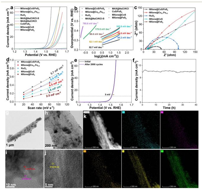
Fig. 5 (a) LSV polarization curves, (b) Tafel slopes, (c) Nyquist plots, and (d)  $C_{\rm cl}$  curves of the catalysts. (e) LSV curves of MXene@CoS/FeS<sub>2</sub> before and after 2000 CV cycles. (f) Chronoamperometric curve of MXene@CoS/FeS<sub>2</sub>. (g, h) TEM, (i, j) HRTEM, and (k) EDS elemental mapping images of MXene@CoS/FeS<sub>2</sub> after the long-term stability test.
