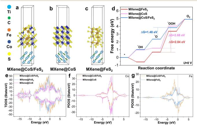
Fig. 6 Schematic models of the optimized (a) MXene@CoS/FeS<sub>2</sub>, (b) MXene@CoS, and (c) MXene@FeS<sub>2</sub>. (d) Calculated OER free-energy diagrams of the catalysts at a potential of 0 V. (e) TDOS curves of the samples. (f, g) PDOS curves of the catalysts.
