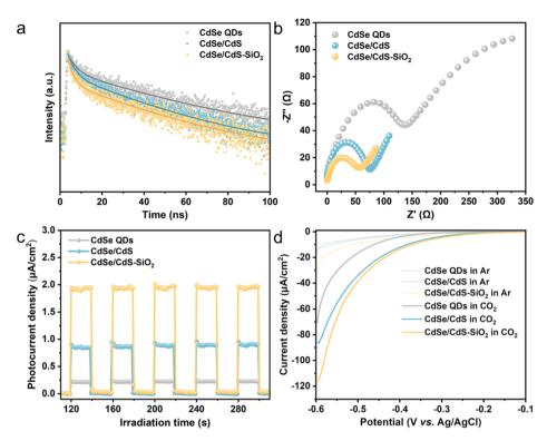
Fig. 4 (a) TRPL decay plots, (b) EIS plots and (c) transient photocurrent spectra of CdSe QDs, CdSe/CdS QDs and CdSe/CdS-SiO $_2$  composites. (d) LSV curves of CdSe QDs, CdSe/CdS QDs and CdSe/CdS-SiO $_2$  composites under Ar or CO $_2$  atmospheres.
