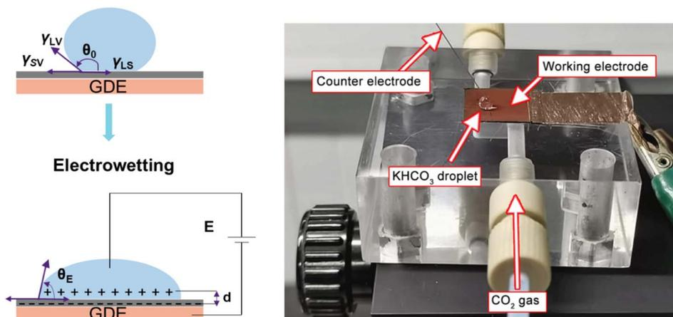
Fig. 5 Illustration of electrowetting (left) and photo of the homemade platform that permits the operando observations of electrowetting during  $\text{CO}_2$  electrolysis developed by Gao *et al.* Adapted from ref. 81 with permission from American Chemical Society, copyright 2021.
