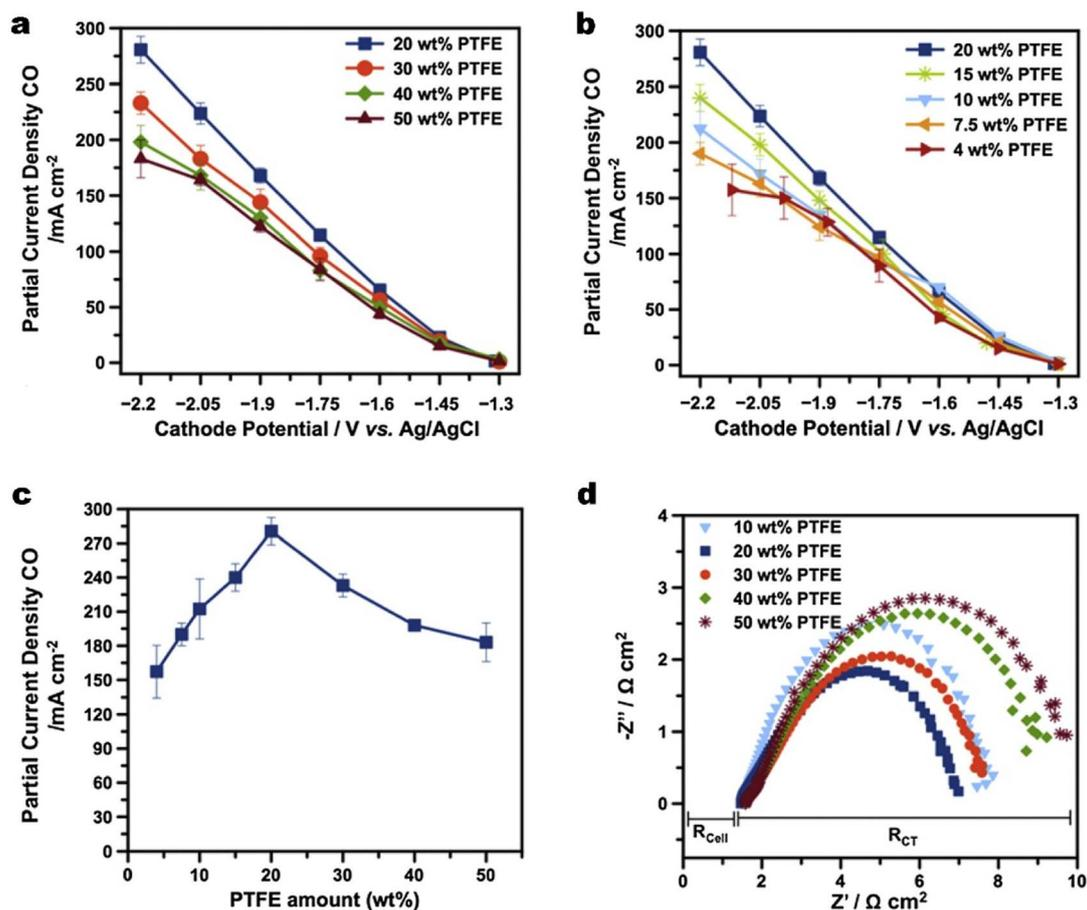
Fig. 11 (a) and (b) Partial current density of CO and H<sub>2</sub> as a function of different potentials for GDEs composed of MPLs with different amounts of PTFE wt%; (c) a comparison of partial current densities of CO for a Ag-based GDE as a function of PTFE content in the MPLs; and (d) the Nyquist plot of electrochemical impedance spectra for the GDEs with different PTFE contents in MPLs. Reproduced from ref. 64 with permission from Elsevier, copyright 2016.
