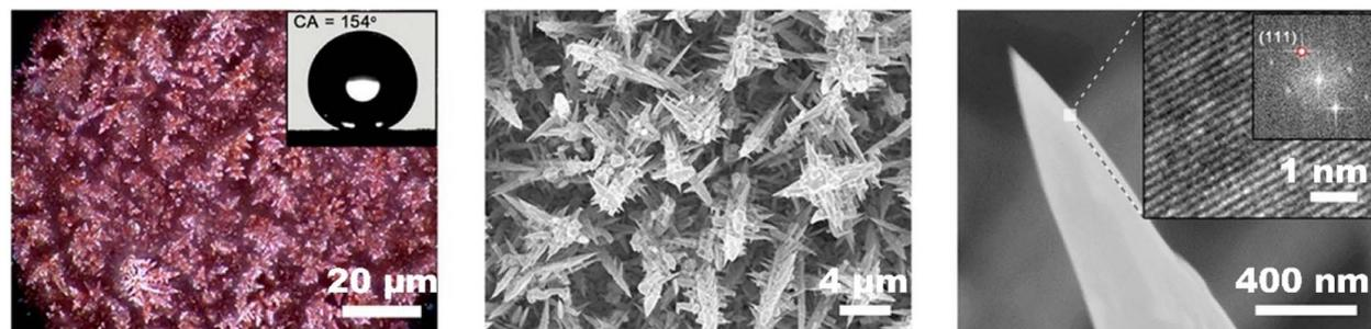
Fig. 10 Tuning the morphology of the catalyst to prevent carbon-based GDEs from being wetted. Reproduced from ref. 81 with permission of American Chemical Society, copyright 2021.
