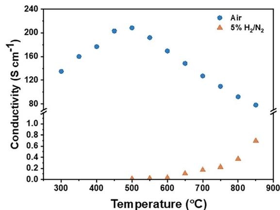
Fig. 4 Conductivity variation of BLFMN with temperature in air and 5% H<sub>2</sub>/N<sub>2</sub>.
