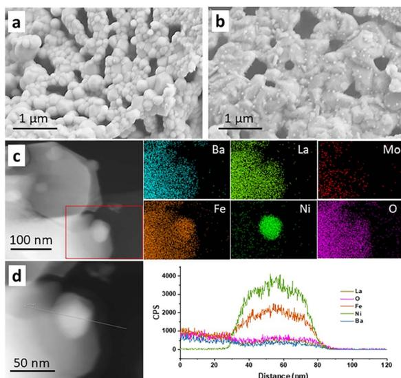
Fig. 2 Surface morphology of the (a) pristine BLFMN powder and (b) BLFMN powder treated in  $\text{H}_2$  at 800 °C for 5 h, (c) HAADF-STEM image and the corresponding EDX element mapping images of an NiFe alloy nanoparticle, and (d) HAADF-STEM image and corresponding EDX line scan of the nanoparticles.
