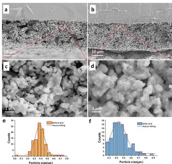
Fig. 9 (a and b) SEM image of the cross section of the fresh cell and the cell after tested with  $\text{CH}_4$ ; (c and d) magnified fractured cross-sectional SEM image of the BLFMN anode for the area in the red rectangle in (a) and (b), respectively; (e and f) the particle size distribution analysis of the fresh BLFMN anode and BLFMN anode after being tested in dry  $\text{CH}_4$  for  $\sim 325 \text{ h}$ , respectively.
