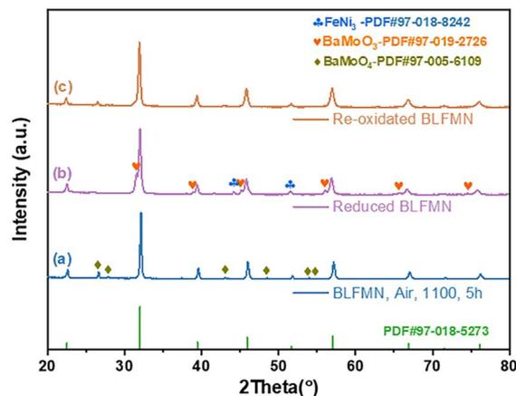
Fig. 1 X-ray diffraction patterns of (a) the as-prepared pristine BLFMN, (b) BLFMN reduced in H<sub>2</sub> at 800 °C for 5 h, and (c) reduced BLFMN being re-oxidized at 800 °C for 5 h in air.
