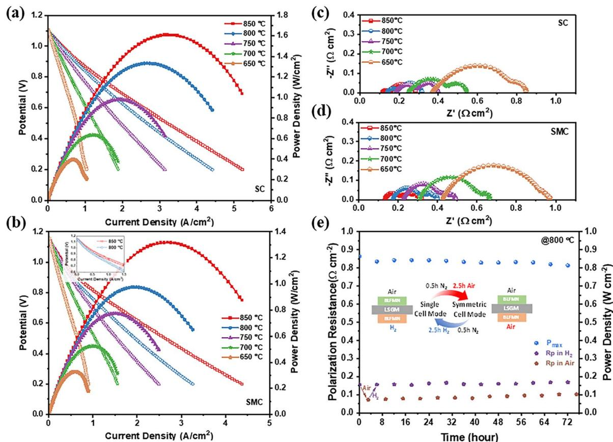
Fig. 6 (a and c)  $I$ - $V$ - $P$  and EIS curves for the BLFMN//LSGM//LSCF single cell (SC) operating from 650 to 850 °C. (b and d)  $I$ - $V$ - $P$  and EIS curves for the BLFMN//LSGM//BLFMN symmetric cell (SMC) operating from 650 to 850 °C. (e) Redox cycling stability of the BLFMN electrode with cell configuration of BLFMN//LSGM//BLFMN at 800 °C between the mode of the symmetric cell and the single cell.
