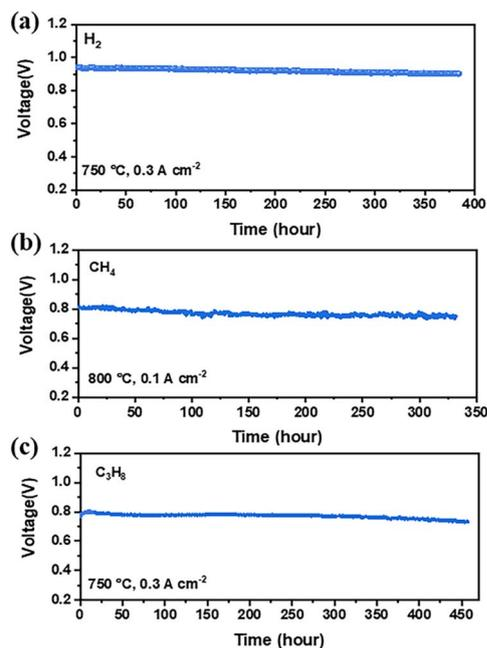
Fig. 8 Performance stability test for the single cells with the BLFMN|LSGM|LSCF configuration under a constant current load of (a)  $0.3 \text{ A cm}^{-2}$  at  $750 \text{ }^\circ\text{C}$  in  $\text{H}_2$ , (b)  $0.1 \text{ A cm}^{-2}$  at  $800 \text{ }^\circ\text{C}$  in  $\text{CH}_4$ , and (c)  $0.3 \text{ A cm}^{-2}$  at  $750 \text{ }^\circ\text{C}$  in  $\text{C}_3\text{H}_8$ .
