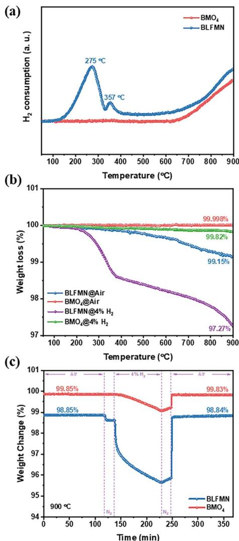
Fig. 3 (a) TPR plot for BLFMN and BMO<sub>4</sub> powders from 50 to 900 °C, (b) TGA in air and 4% H<sub>2</sub>/N<sub>2</sub> for BLFMN and BMO<sub>4</sub> powders from 50 to 900 °C, and (c) weight change of BLFMN and BMO<sub>4</sub> powders by switching the gas between air and 4% H<sub>2</sub>/N<sub>2</sub>; N<sub>2</sub> was purged to the chamber for 20 min to swap the remaining air or 4% H<sub>2</sub>/N<sub>2</sub> for each gas switching.
