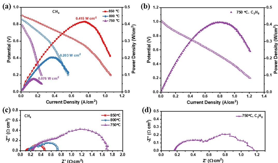
Fig. 7 (a)  $I-V-P$  and (c) EIS curves for the single cell operating from 750 to 850  $^{\circ}C$  with  $CH_4$  as fuel. (b)  $I-V-P$  and (d) EIS curves for the single cell operating at 750  $^{\circ}C$  with  $C_3H_8$  as fuel.
