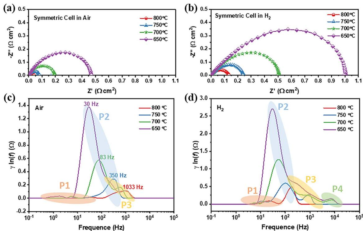
Fig. 5 Electrochemical impedance spectra of BLFMN symmetric cells measured in air (a) and  $\text{H}_2$  (b) at 650, 700, 750, and 800 °C, respectively. Resulting DRT plots of the BLFMN symmetric cell under air (c) and  $\text{H}_2$  (d) atmospheres at 650, 700, 750, and 800 °C, respectively.
