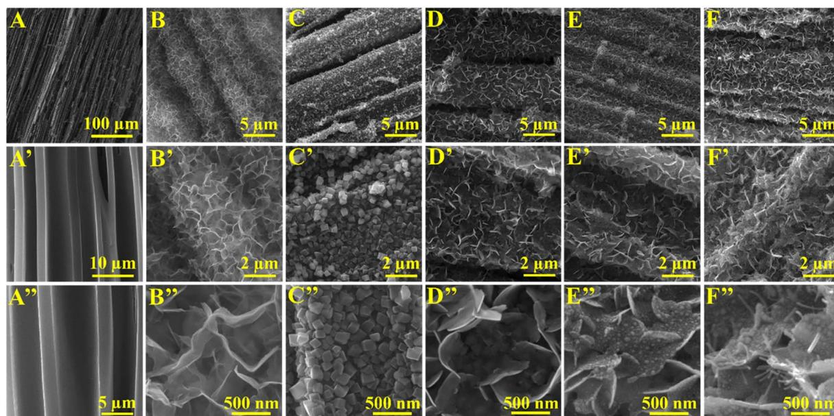
Fig. 2 SEM images of (A–A'') naked NCW, (B–B'') Ni(OH)<sub>2</sub>@NCW, (C–C'') CF@NCW, (D–D'') Ni(OH)<sub>2</sub>-CF@NCW, (E–E'') NS-CF@NCW and (F–F'') NSP-CF@NCW at different magnifications.
