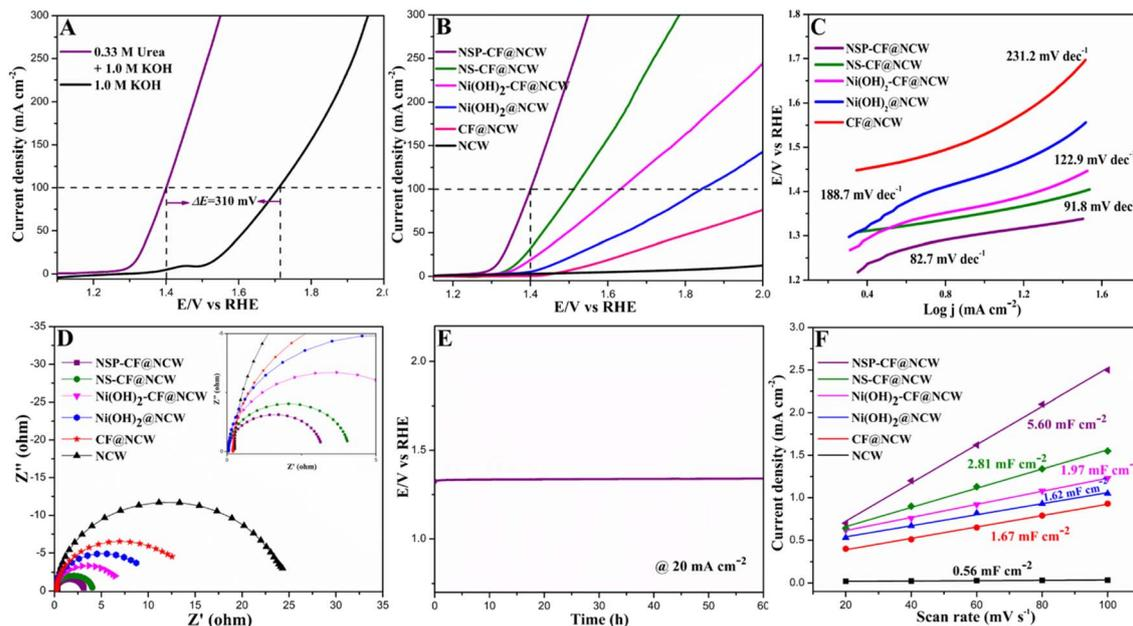
Fig. 5 (A) LSV curves for the OER and UOR of NSP-CF@NCW in 1.0 M KOH and 0.33 M urea + 1.0 M KOH at a scan rate of  $5 \text{ mV s}^{-1}$ . (B) UOR LSVs of all the studied NCWs, (C) the related Tafel slopes, (D) and Nyquist profiles of all the fabricated electrodes in 0.33 M urea + 1.0 M KOH. (E) Chronopotentiometric profile of NSP-CF@NCW at  $20 \text{ mA cm}^{-2}$  in 0.33 M urea + 1.0 M KOH. (F)  $C_{dl}$  values of all the studied anodes.
