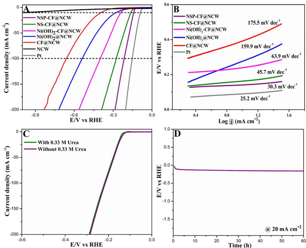
Fig. 6 (A) LSV curves for the HER of all the studied NCWs at a scan rate of  $5 \text{ mV s}^{-1}$  and (B) the related Tafel slopes. (C) LSVs of the NSP-CF@NCW cathode in  $1.0 \text{ M KOH}$  and  $0.33 \text{ M urea} + 1.0 \text{ M KOH}$ . (D) Chronopotentiometric plot of the NSP-CF@NCW cathode at  $20 \text{ mA cm}^{-2}$  for the HER.
