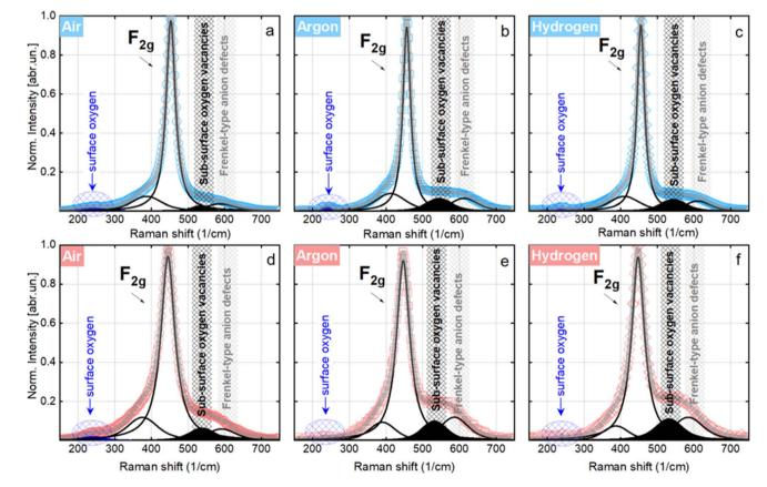
Fig. 3 Raman spectra of Ni/CeO<sub>2-x</sub> catalysts calcined in different atmospheres at room temperature (blue data) and 500 °C (red data) in an equimolar  $CH_4/CO_2$  flow, accompanied by Gaussian peak deconvolution.
