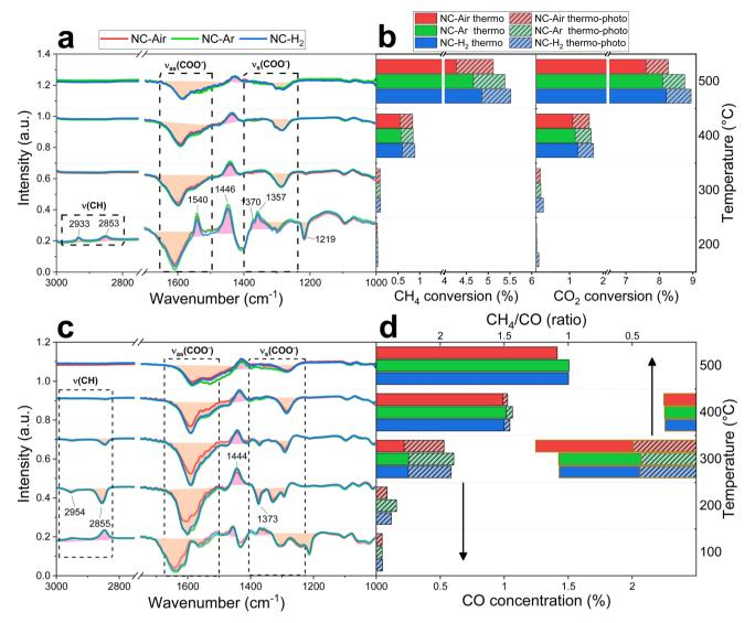
Fig. 4 Difference spectra between thermal and photo-thermal conditions during operando DRM (a) and RWGS (c), combined with the measured  $CH_4$  and  $CO_2$  conversions for DRM reactions (b), and (d) CO concentration and the  $CH_4/CO$  ratio during the RWGS reaction.
