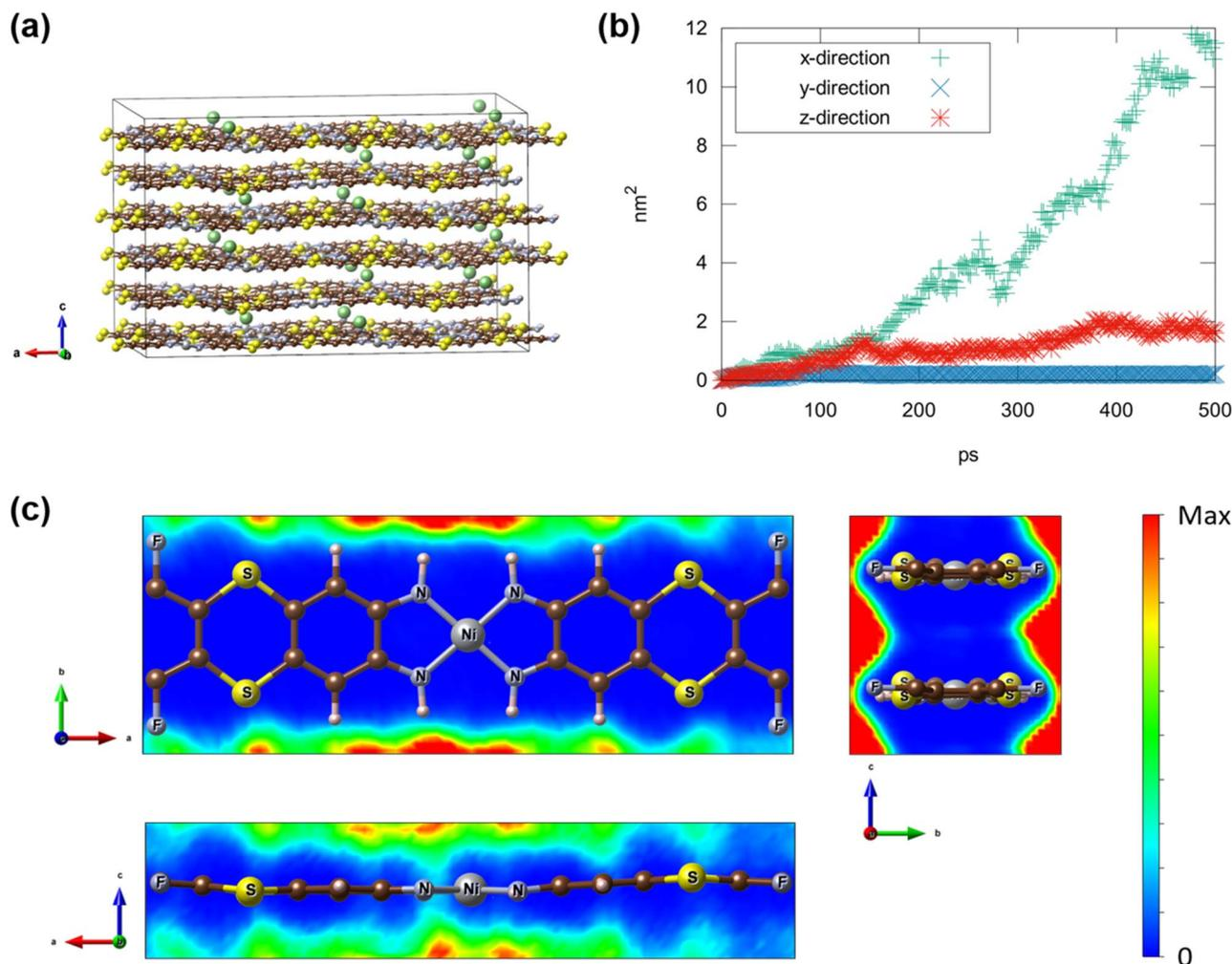
Fig. 5 Molecular dynamics (MD) simulation of SKIER-5. (a) Initial structure of the Li-intercalated SKIER-5 ( $\text{Li}_{24}\text{C}_{864}\text{S}_{192}\text{F}_{96}\text{N}_{192}\text{H}_{384}\text{Ni}_{48}$ ) for the molecular dynamics simulation and (b) the calculated mean squared displacement (MSD) over 500 ps at 300 K. (c) The population density map of the relative positions of Li ions from each Ni site in SKIER-5.
