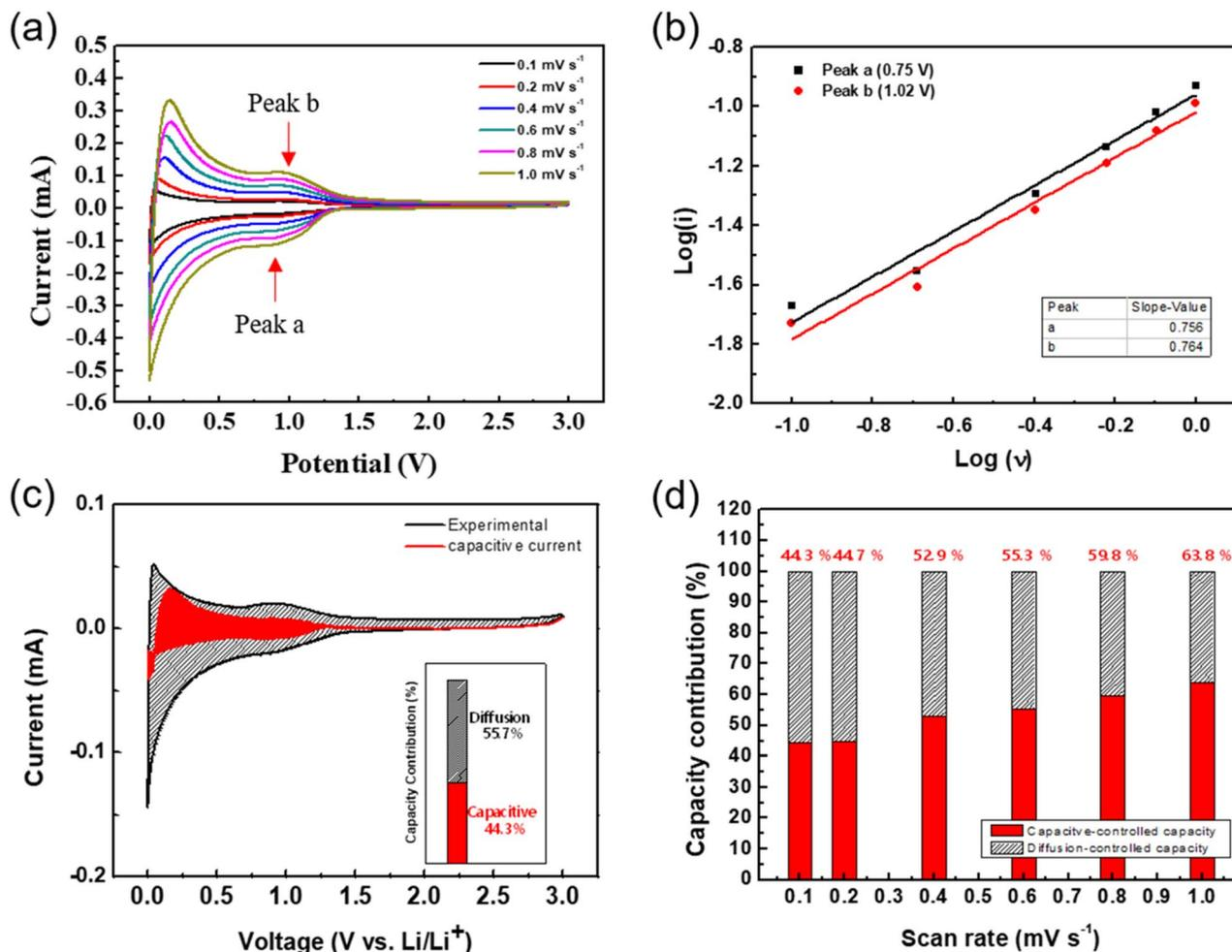
Fig. 3 Dunn method analysis of SKIER-5. (a) CV curves obtained at different scan rates. (b) The corresponding  $\log(i)$  versus  $\log(v)$  plots for the two peaks in the CV scans of panel a. (c) Capacitive contribution (red area) at a scan rate of  $0.1 \text{ mV s}^{-1}$ . (d) Ratio of capacitive contribution (red) at various scan rates.
