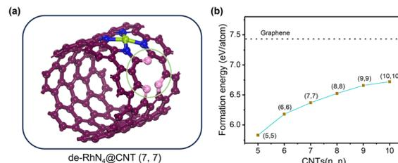
Fig. 5 Defect formation energies as a function of  $n$  of CNTs. (a) Optimized structure of  $\text{de-RhN}_4@\text{CNTs}$  ( $7, 7$ ) with a 5-1DB defect. (b) The formation energy of a 5-1DB defect on graphene and  $\text{RhN}_4@\text{CNTs}$  ( $n, n$ ) ( $n = 5-10$ ).
