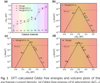
Fig. 1 DFT-calculated Gibbs free energies and volcano plots of the exchange current density. (a) Gibbs free energy of H adsorption ( $\Delta G_{H^*}$ ) on TMN<sub>4</sub>@C and TMN<sub>4</sub>@CNTs (n, n) (n = 5, 10), TM = Mo, Ru, Rh, Fe, Cr, Co, Ag, Zn, Mn, Cu, Ni, Pd. (b)–(d) Volcano plot between exchange current density  $(i_0)$  and  $\Delta G_{H^*}$  in TMN<sub>4</sub>@CNTs (n, n) (n = 5, 10) and TMN<sub>4</sub>@C. Data for the Pt (111) surface were obtained from ref. 32.
