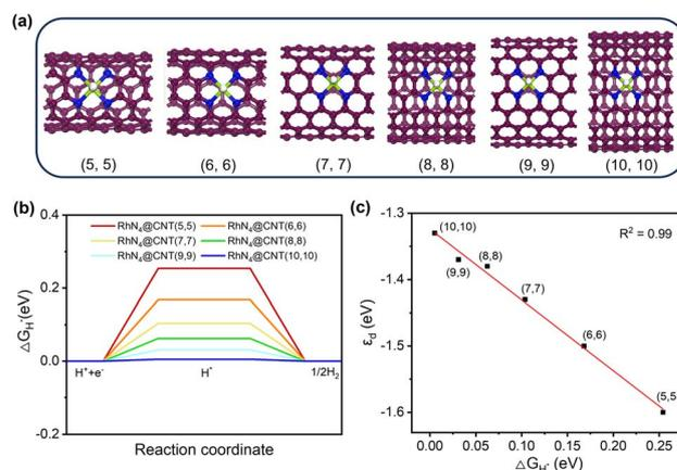
Fig. 3 HER activity of  $\text{RhN}_4@CNTs$  with six different curvatures. (a) Optimized geometric model of  $\text{RhN}_4@CNTs$  ( $n, n$ ) ( $n = 5-10$ ) adsorbed with a single H atom. (b)  $\Delta G_{H^*}$  on  $\text{RhN}_4@CNTs$  ( $n, n$ ) ( $n = 5-10$ ). (c) Correlation between  $\Delta G_{H^*}$  and d-band center ( $\epsilon_d$ ) of Rh anchored on CNTs with different nanotube diameters.
