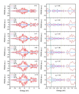
Fig. 4 Partial density of states (PDOS) for RhN<sub>4</sub>@CNTs (n, n) (n = 5– 10), C-state, N-state, and Rh-state are represented by red, purple, and blue. On the right is an enlarged view in the energy range of -2 to 2 eV. The dotted line and the full line represent the position of the Fermi level and d-band center ( $\varepsilon_d$ ), respectively.
