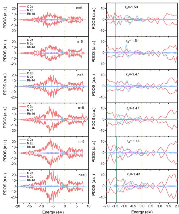
Fig. 7 PDOS for de-RhN<sub>4</sub>@CNTs (*n*, *n*) (*n* = 5–10). C-state, N-state, and Rh-state are represented by red, purple, and blue. The right is an enlarged view in the energy range of –2 to 2 eV. The dotted line and the full line represent the position of the Fermi level and d-band center ( $\epsilon_d$ ), respectively.
