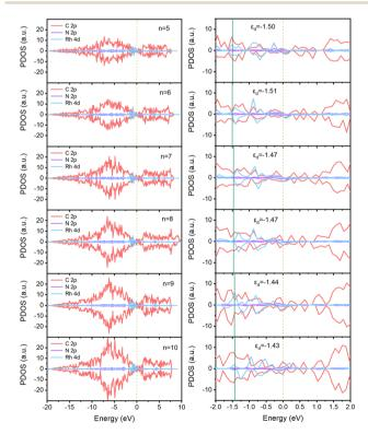
Fig. 7 PDOS for de-RhN<sub>4</sub>@CNTs (n, n) (n = 5-10), C-state, N-state, and Rh-state are represented by red, purple, and blue. The right is an enlarged view in the energy range of -2 to 2 eV. The dotted line and the full line represent the position of the Fermi level and d-band center  $(\varepsilon_d)$ , respectively.
