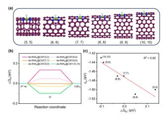
Fig. 6 HER activity of de-RhN<sub>4</sub>@CNTs with six different curvatures. (a) Optimized geometric model of de-RhN<sub>4</sub>@CNTs (n, n) (n = 5-10)adsorbed with hydrogen. (b) Calculated Gibbs free energy  $\Delta G_{H^*}$  on de-RhN<sub>4</sub>@CNTs (n, n) (n = 5-10). (c) Correlation between  $\Delta G_{H^*}$  and dband center ( $\varepsilon_d$ ).
