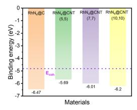
Fig. 2 The calculated cohesive energy of Rh and the binding energy  $(E_{\rm b})$  of RhN<sub>4</sub>@C and RhN<sub>4</sub>@CNTs (n,n) (n=5,7,10).
