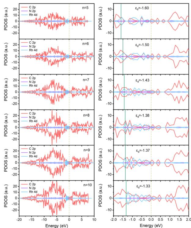
Fig. 4 Partial density of states (PDOS) for  $\text{RhN}_4@\text{CNTs}$  ( $n, n$ ) ( $n = 5-10$ ). C-state, N-state, and Rh-state are represented by red, purple, and blue. On the right is an enlarged view in the energy range of  $-2$  to  $2$  eV. The dotted line and the full line represent the position of the Fermi level and d-band center ( $\epsilon_d$ ), respectively.
