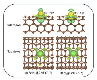
Fig. 8 Bader charge, and charge density difference for H atom adsorption on RhN<sub>4</sub>@CNTs (7, 7) and de-RhN<sub>4</sub>@CNTs (7, 7). The yellow region represents charge accumulation, and the cyan region represents charge depletion. The isosurface value is 0.002 e bohr<sup>-3</sup>
