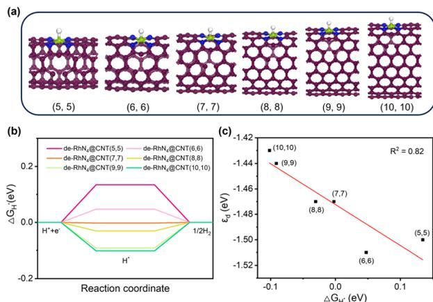
Fig. 6 HER activity of de-RhN<sub>4</sub>@CNTs with six different curvatures. (a) Optimized geometric model of de-RhN<sub>4</sub>@CNTs (*n*, *n*) (*n* = 5–10) adsorbed with hydrogen. (b) Calculated Gibbs free energy  $\Delta G_{H^*}$  on de-RhN<sub>4</sub>@CNTs (*n*, *n*) (*n* = 5–10). (c) Correlation between  $\Delta G_{H^*}$  and d-band center ( $\epsilon_d$ ).
