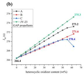
Fig. 5 (a) Calculated  $l_{sp}$  values of HTPB propellants (AP + 18% aluminium + 14% HTPB + heterocyclic oxidizer) at different heterocyclic oxidizer contents. (b) Calculated  $I_{sp}$  values of GAP propellants (AP + 18% aluminium + 20% GAP + heterocyclic oxidizer) at different heterocyclic oxidizer
