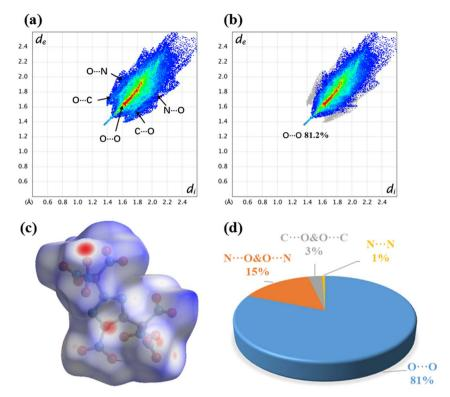
Fig. 3 (a) 2D fingerprint plots in crystal packing found in JY-23. (b) O···O atomic contact percentage contribution to the Hirshfeld surface for JY-23. (c) Hirshfeld surface graph of JY-23. (d) Percentage contributions of the individual atomic contacts to the Hirshfeld surface for JY-23.
