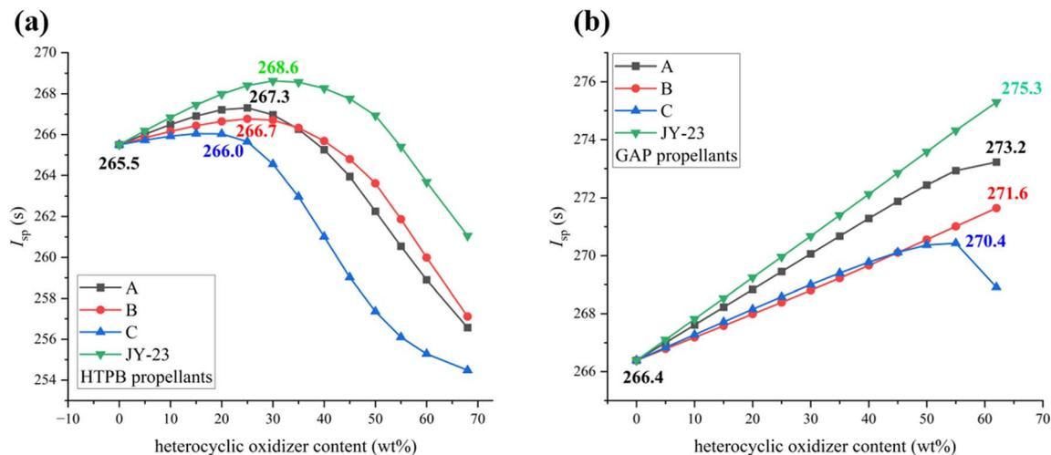
Fig. 5 (a) Calculated  $I_{sp}$  values of HTPB propellants (AP + 18% aluminium + 14% HTPB + heterocyclic oxidizer) at different heterocyclic oxidizer contents. (b) Calculated  $I_{sp}$  values of GAP propellants (AP + 18% aluminium + 20% GAP + heterocyclic oxidizer) at different heterocyclic oxidizer contents.
