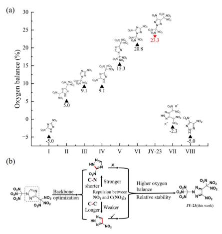
(a) The oxygen balance comparison of JY-23 with other nitro-triazole compounds. (b) The design of molecular stability
