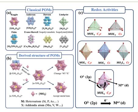
Fig. 1 (a) Polyhedral structure view of classical POM types. (b) Conversion of Keggin-type POM derivative system. (c) Different types of the polyhedral MO<sub>x</sub>L<sub>v</sub> of POMs and redox activities in POM structural unit.
