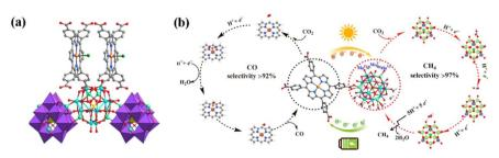
Fig. 6 (a) Crystal structures of M-POMOFs. (b) Proposed reaction mechanism in PCR and ECR (photo- and electrocatalytic  $CO_2$  reduction) reactions for Fe-POMOF, respectively. Reproduced from ref. 115. Copyright 2022, The Authors, some rights reserved; exclusive licensee American Association for the Advancement of Science.
