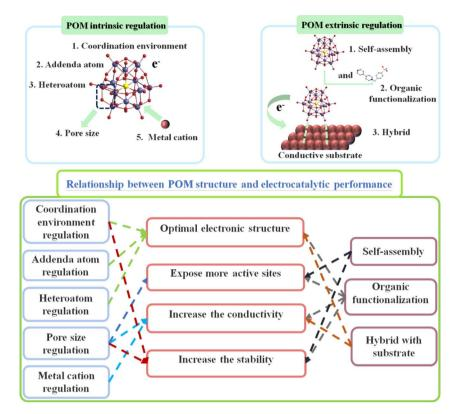
Scheme 1 Relationship between structure control strategy and electrocatalytic performance of POM-based electrocatalysts.
