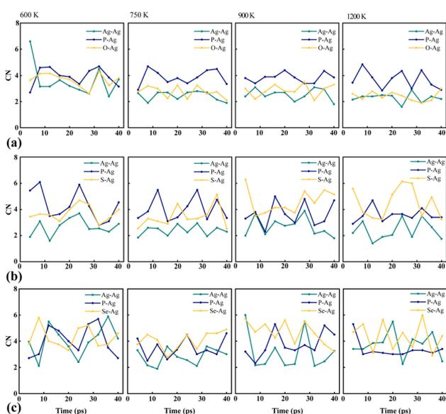
**Fig. 7** Calculated average coordination numbers (CNs) for Ag as the central atom, with P, O, S, and Se as neighboring atoms, are presented for (a)  $\text{Ag}_7\text{P}_3\text{O}_{11}$ , (b)  $\text{Ag}_7\text{P}_3\text{S}_{11}$ , and (c)  $\text{Ag}_7\text{P}_3\text{Se}_{11}$ . These CNs illustrate the distribution of formation pairs involving Ag with each type of neighbor atom.
