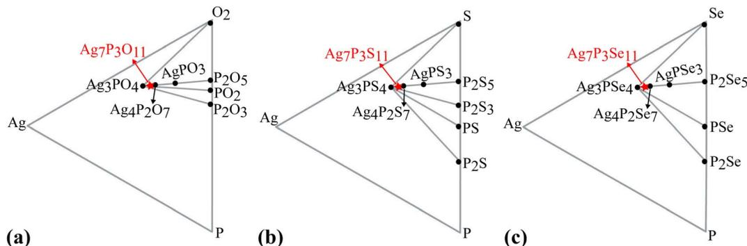
Fig. 5 Phase evolution of (a)  $\text{Ag}_7\text{P}_3\text{O}_{11}$ , (b)  $\text{Ag}_7\text{P}_3\text{S}_{11}$ , and (c)  $\text{Ag}_7\text{P}_3\text{Se}_{11}$  is analyzed. For all compositions, the equilibrium state is determined by a combination of stable phases found within the linear and triangular surroundings of each composition. The position of each  $\text{Ag}_7\text{P}_3\text{X}_{11}$  compound within this phase space is indicated by a red star.
