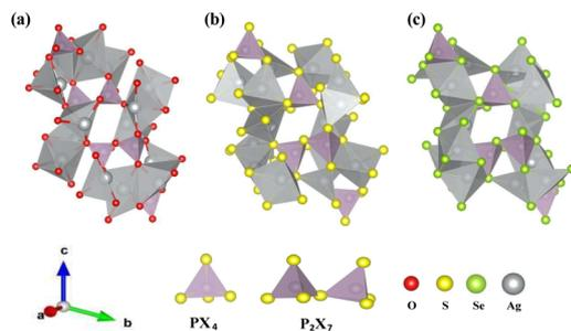
Fig. 1 The relaxed crystal structures of (a)  $\text{Ag}_7\text{P}_3\text{O}_{11}$ , (b)  $\text{Ag}_7\text{P}_3\text{S}_{11}$ , and (c)  $\text{Ag}_7\text{P}_3\text{Se}_{11}$  are presented. These crystals each possess a triclinic structure and belong to the space group  $P1$ .
