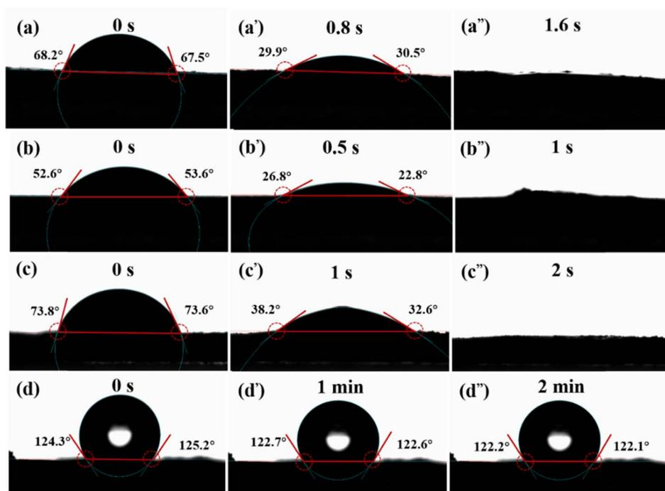
Fig. 5 Wettability measurements: dynamic contact angle for the water droplet on (a–a'') VAGNA-S-1000, (b–b'') VAGNA-T-1000, (c–c'') VAGNA-L-1000, and (d–d'') the control sample-VAGNA *via* the PECVD method.
