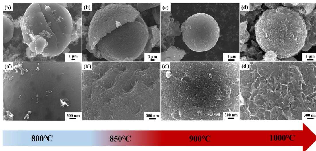
Fig. 8 Low- and high-magnification FE-SEM images of hydrothermal-treated lotus pollen-derived VAGNAs pyrolyzed with  $K_2CO_3$  at different temperatures: (a and a') 800 °C, (b and b') 850 °C, (c and c') 900 °C and (d and d') 1000 °C.
