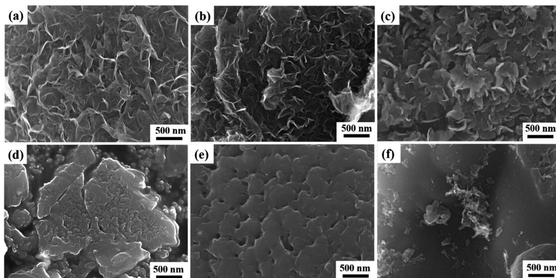
Fig. 7 FE-SEM images of lotus pollen-derived carbons *via* HSP method using different salts at 1000 °C: (a)  $\text{K}_2\text{CO}_3$ , (b)  $\text{CH}_3\text{COOK}$ , (c)  $\text{Na}_2\text{CO}_3$ , (d)  $\text{Li}_2\text{CO}_3$ , (e) KCl and (f)  $\text{K}_3\text{PO}_4$ .
