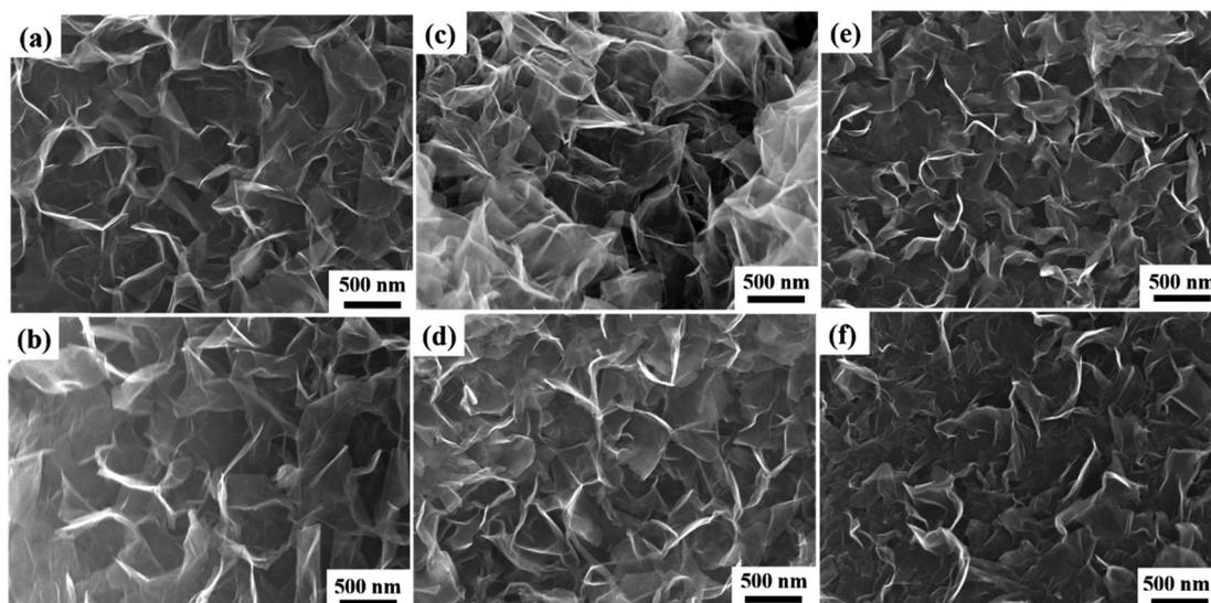
Fig. 2 FE-SEM images of VAGNAs from the pyrolysis of different biomasses with  $K_2CO_3$  at 1000 °C: (a) VAGNA-S-1000, (b) VAGNA-G-1000, (c) VAGNA-T-1000, (d) VAGNA-P-1000, (e) VAGNA-L-1000 and (f) VAGNA-R-1000.
