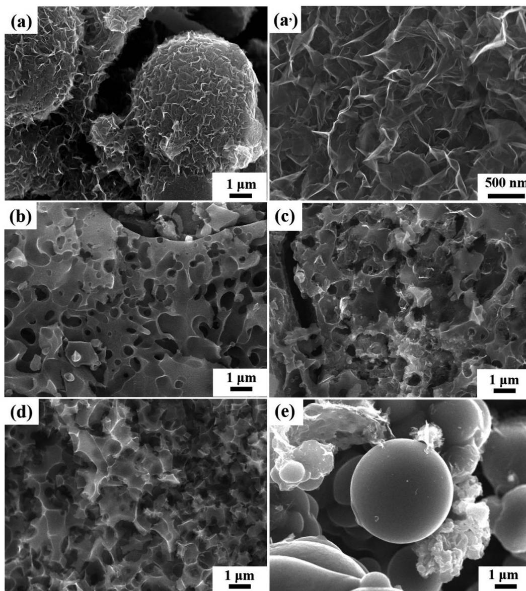
Fig. 6 FE-SEM images of lotus pollen-derived carbons (VAGNA) from pretreated precursors with different methods. (a and a'): hydrothermal treatment, (b) NaOH soaking, (c) H<sub>2</sub>SO<sub>4</sub> soaking, (d) ammonia soaking and (e) without pretreatment.
