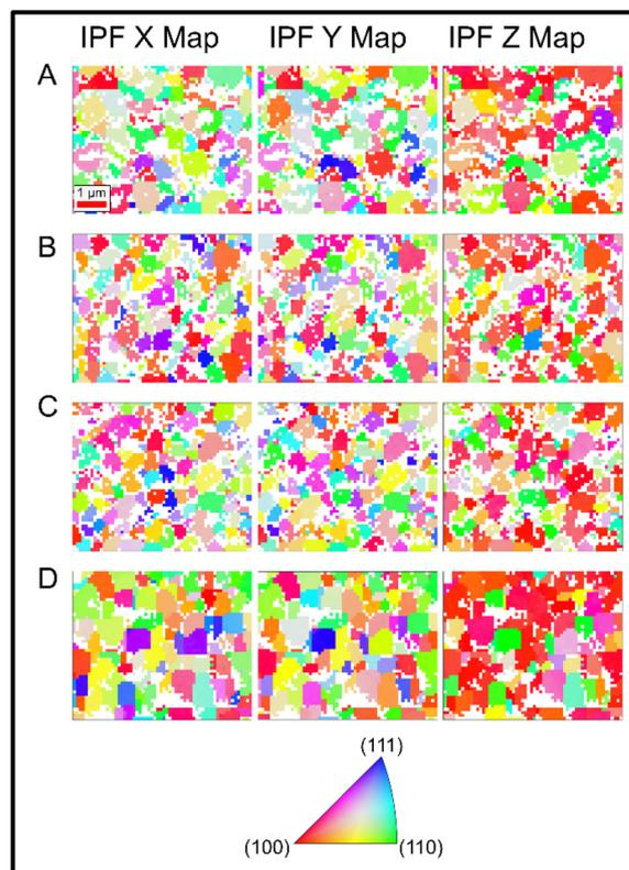
Fig. 2 IPF maps showing grain level crystallographic orientation for  $\text{PbCl}_2$  doped  $\text{CsPbI}_2\text{Br}$  films – (A) 0%,  $0 \text{ mg mL}^{-1}$ , (B) 1%,  $1.8 \text{ mg mL}^{-1}$ , (C) 3%,  $5.0 \text{ mg mL}^{-1}$ , and (D) 5%,  $8.4 \text{ mg mL}^{-1}$ .
