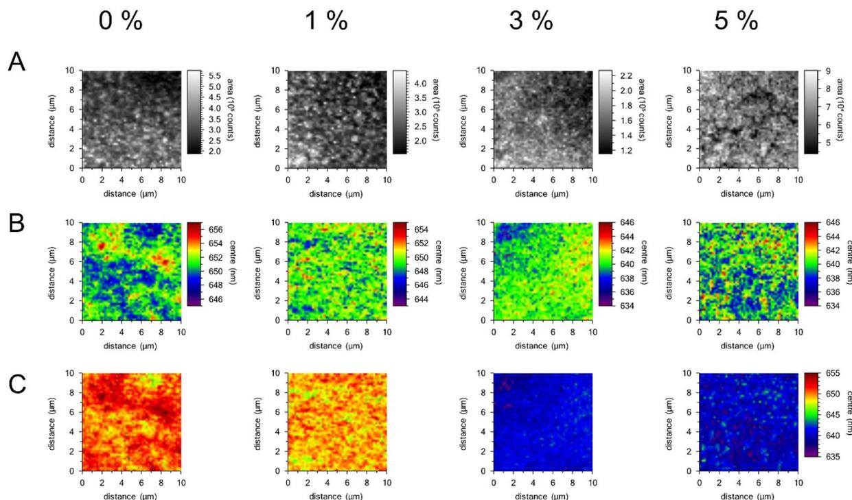
Fig. 6 (A) Integrated intensity CL plots of the samples, (B) centroid wavelength plots displaying peak position changes within the samples, (C) centre wavelength plots all on the same wavelength scale.
