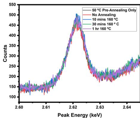
Fig. 8 WDX peak for chlorine within a 5%  $\text{PbCl}_2$  doped sample, showing the effect of annealing time [pre-annealing for 2 minutes at 50 °C followed by 10, 30 and 60 minutes at 160 °C] on peak intensity.
