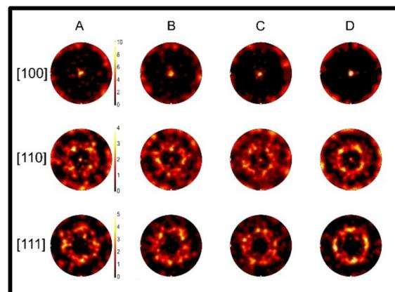
Fig. 3 Pole figures for the [100], [110] and [111] directions measured for the samples using EBSD (A) 0%,  $0 \text{ mg mL}^{-1}$ , (B) 1%,  $1.8 \text{ mg mL}^{-1}$ , (C) 3%,  $5.0 \text{ mg mL}^{-1}$ , and (D) 5%,  $8.4 \text{ mg mL}^{-1}$  [undoped and doped (1, 3 and 5%  $\text{PbCl}_2$ )  $\text{CsPbI}_2\text{Br}$  films]. The scales (counts) are the same along each row.
