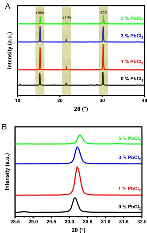
Fig. 1 (A) XRD pattern for undoped and doped (1, 3 and 5%  $\text{PbCl}_2$ )  $\text{CsPbI}_2\text{Br}$  films (B) magnified view showing shift in the (200) peak position with increase in dopant concentration.
