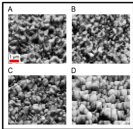
Fig. 4 Band contrast maps for the sample set, pattern signal on intensity scale.  $\text{PbCl}_2$  doped  $\text{CsPbI}_2\text{Br}$  (A) 0%,  $0 \text{ mg ml}^{-1}$ , (B) 1%,  $1.8 \text{ mg ml}^{-1}$ , (C) 3%,  $5.0 \text{ mg ml}^{-1}$ , and (D) 5%,  $8.4 \text{ mg ml}^{-1}$ .
