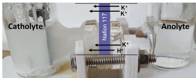
Fig. 5 H-cell picture showing the precipitate formation on the catholyte side after the CO<sub>2</sub>RR in dry acetonitrile and KOH (0.5 M) as the anolyte.
