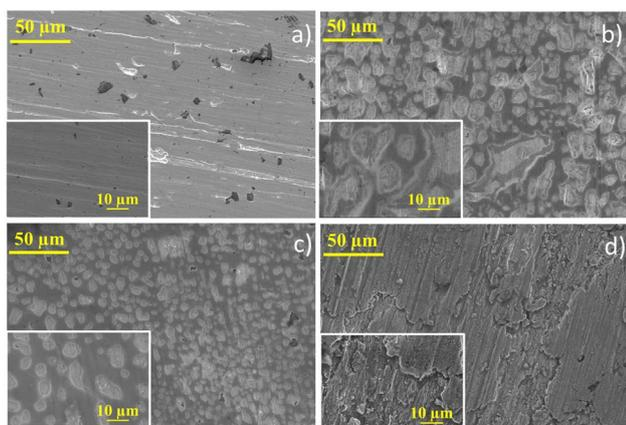
Fig. 3 Scanning electron microscopy images for (a) cleaned Pb plate before the reaction and for the Pb plate after the reaction using (b) acidic anolyte (H<sub>2</sub>SO<sub>4</sub>), (c) near-neutral anolyte (KHCO<sub>3</sub>), and (d) alkaline anolyte (KOH).
