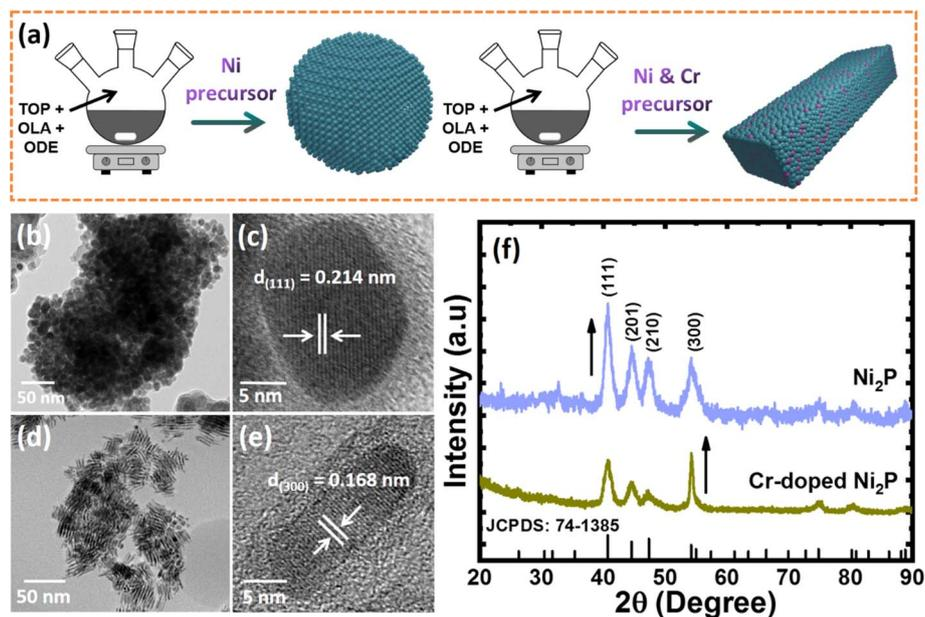
Fig. 1 (a) Schematic illustration of the synthesis process, (b and c) high resolution TEM and HR-TEM images of  $\text{Ni}_2\text{P}$ , (d and e) high resolution TEM and HR-TEM images of  $\text{Ni}_{1.2}\text{Cr}_{0.8}\text{P}$ , and (f) their corresponding PXRD patterns.
