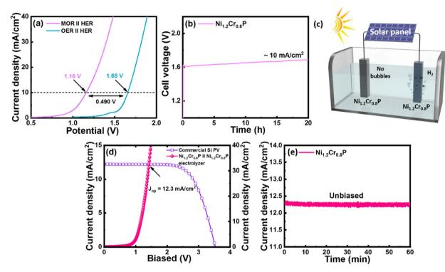
Fig. 5 (a) Comparison of polarization curves for OMeS (MOR $\parallel$ HER) in 1.0 M KOH/3 M MeOH and OWS (OER $\parallel$ HER) in 1 M KOH using Ni<sub>1.2</sub>Cr<sub>0.8</sub>P electrocatalysts as both an anode and a cathode. (b) Long-term durability test of OMeS for 20 h. (c) Schematic representation of a solar-driven electrolysis cell. (d) Solar-to-hydrogen (STH) efficiency plot for the OMeS system (e) Unbiased water splitting photocurrent measured for 60 min in the OMeS system.
