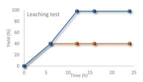
Fig. 6 Reaction profile with or without the catalyst (after separating the catalyst from the reaction mixture via hot-filtration technique)
