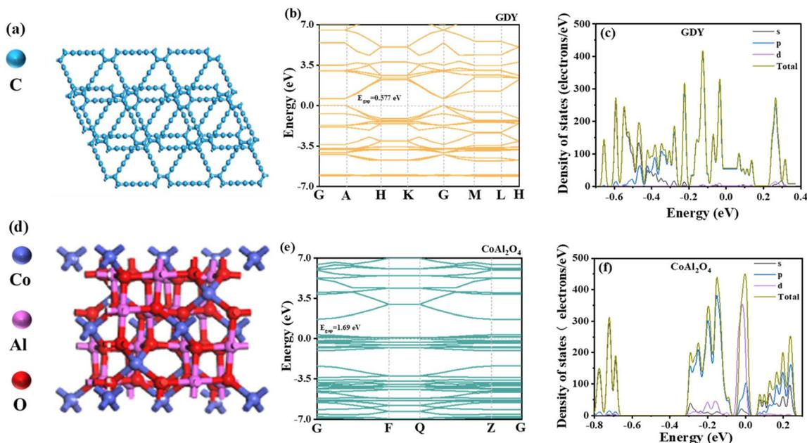
Fig. 13 (a and d) The unit cell of GDY and  $\text{CoAl}_2\text{O}_4$ ; (b and e) band structure of GDY and  $\text{CoAl}_2\text{O}_4$ ; (c and f) densities of states of GDY and  $\text{CoAl}_2\text{O}_4$ .
