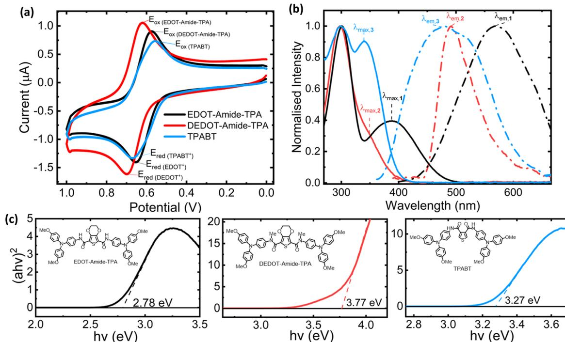
Fig. 1 (a) Cyclic voltammograms referenced to the  $\text{Fc}/\text{Fc}^+$  redox couple ( $\text{CH}_2\text{Cl}_2$ ,  $1 \times 10^{-4}$  M), (b) solution UV-visible absorption (solid lines) and emission spectra (dashed lines) of the three amide-based HTMs, and (c) Tauc plots and corresponding optical bandgaps  $E_g$ .
