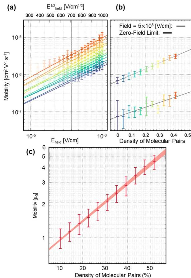
Fig. 10 (a) Mobility against field at different pair densities, (b) mobility against pair density at a field strength of  $5 \times 10^5$  V cm<sup>-1</sup> and at zero field, (c) normalised mobility against pair density.
