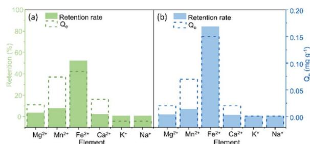
Fig. 3 Adsorption selectivity test of (a) **TAPB-PDA-COF**, and (b) **TAPB-DHTA-COF** in the presence of other cations:  $\text{Ca}^{2+}$ ,  $\text{Mg}^{2+}$ ,  $\text{Mn}^{2+}$ ,  $\text{Na}^+$ ,  $\text{Fe}^{2+}$ , and  $\text{K}^+$ .  $C_{\text{Ca}} = 1.715$  ppm,  $C_{\text{Mg}} = 0.982$  ppm,  $C_{\text{Mn}} = 1.095$  ppm,  $C_{\text{Na}} = 0.376$  ppm,  $C_{\text{Fe}} = 0.177$  ppm, and  $C_{\text{K}} = 0.283$  ppb.
