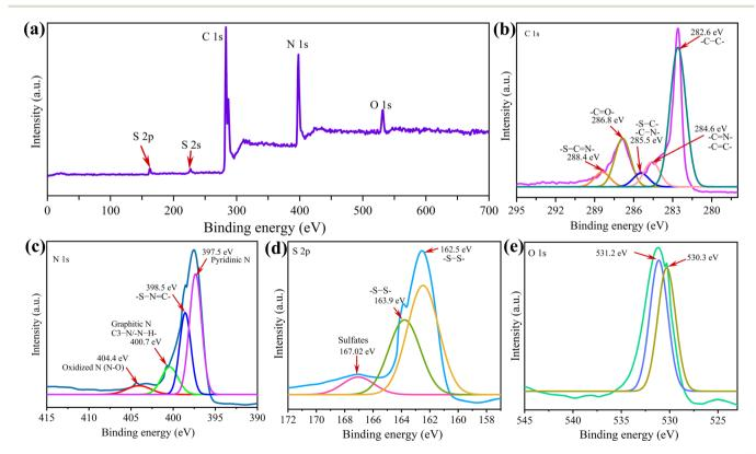
Fig. 2 (a) XPS spectrum showing the complete scan and the corresponding spectra for the elements (b−e) present in the g-C<sub>3</sub>N<sub>4</sub>-CNT/S composite.
