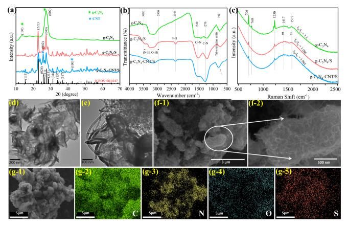
Fig. 1 For  $q-C_3N_4$ ,  $q-C_3N_4/S$ , and  $q-C_3N_4-CNT/S$ : (a) XRD patterns, (b) FTIR spectra and (c) Raman spectra; TEM images for (d)  $q-C_3N_4$  and (e)  $q-C_3N_4$  $C_3N_4$ -CNT/S materials; (f) SEM images for g- $C_3N_4$ -CNT/S; (g) color mapping of g- $C_3N_4$ -CNT/S demonstrating the uniform distribution of C, N, O. and S elements.
