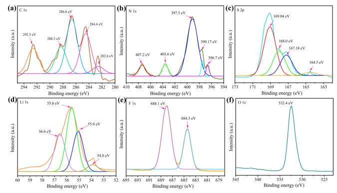
Fig. 8 (a-f) XPS spectra of the  $q-C_3N_4$ -CNT/S cathode obtained from the pouch cell cycled for 250 charge-discharge cycles.
