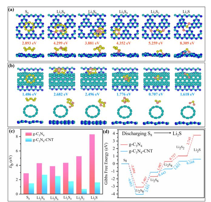
Fig. 4 Optimized configurations of LiPSs on the surfaces of (a) g-C<sub>3</sub>N<sub>4</sub> and (b) the heterostructure of g-C<sub>3</sub>N<sub>4</sub>-CNT. The yellow, pink, cyan, and blue spheres represent sulfur (S), lithium (Li), carbon (C), and nitrogen (N) atoms, respectively. Panel (c) displays the binding energies and panel (d) illustrates the relative free energy for the discharging process from  $S_8$  to  $Li_2S$  on both  $g-C_3N_4$  and  $g-C_3N_4-CNT$  surfaces.
