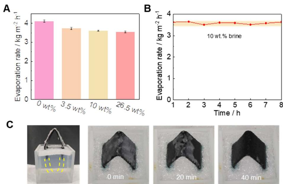
Fig. 4 Salt accumulation evaluation. (A) Daytime evaporation performance of the dual-side 3D evaporator in 3.5, 10, and 26.5 wt% brines; (B) evaporation rates of the 3D evaporator in 10 wt% brine for 8 hours under one sun; (C) salt accumulation evaluation of the 3D dual-side evaporator due to the quick salt ion diffusion process.
