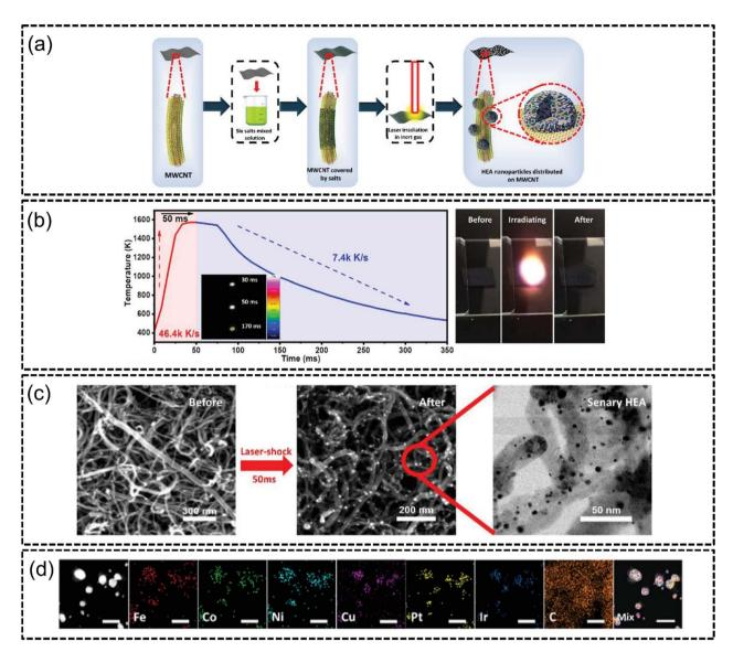
Fig. 8 Laser irradiation synthesis of FeCoNiCuPtlr HEA on MWCNTs from the work of Lu *et al.*, (a) illustration of sample preparation, (b) temperature—time measurements of the duration of laser irradiation of a specific laser spot, (c) FESEM images of salt precursors on MWCNTs before and after laser irradiation, and (d) STEM-EDX elemental mapping of the HEA elements. The scale is 10 nm. Reproduced with permission. Copyright Wiley-VCH GmbH 2022.
