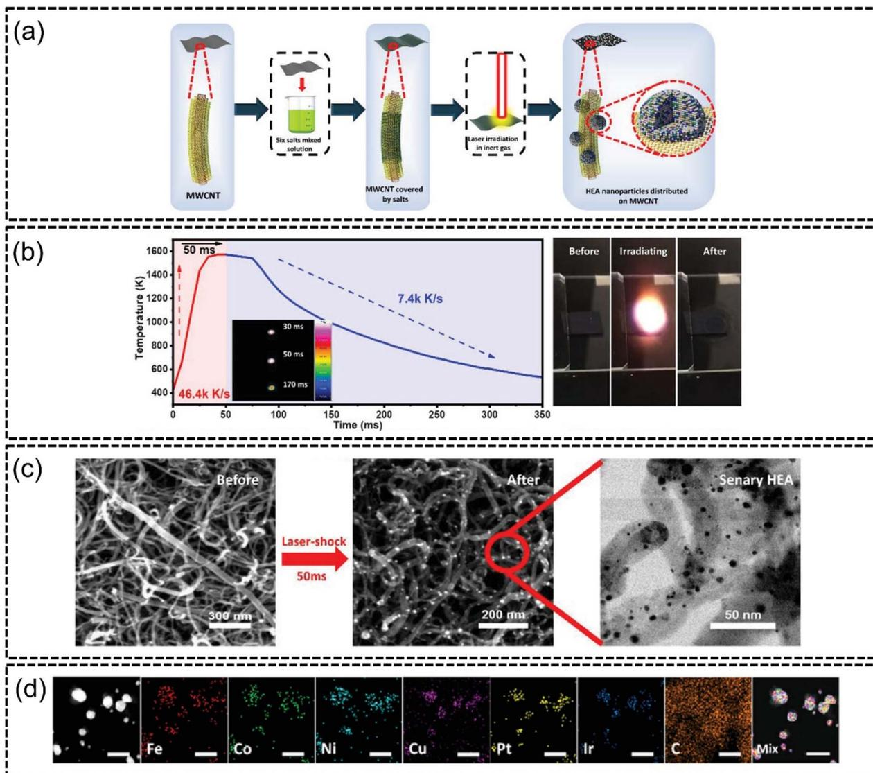
Fig. 8 Laser irradiation synthesis of FeCoNiCuPtIr HEA on MWCNTs from the work of Lu *et al.*, (a) illustration of sample preparation, (b) temperature–time measurements of the duration of laser irradiation of a specific laser spot, (c) FESEM images of salt precursors on MWCNTs before and after laser irradiation, and (d) STEM-EDX elemental mapping of the HEA elements. The scale is 10 nm. Reproduced with permission.<sup>115</sup> Copyright Wiley-VCH GmbH 2022.
