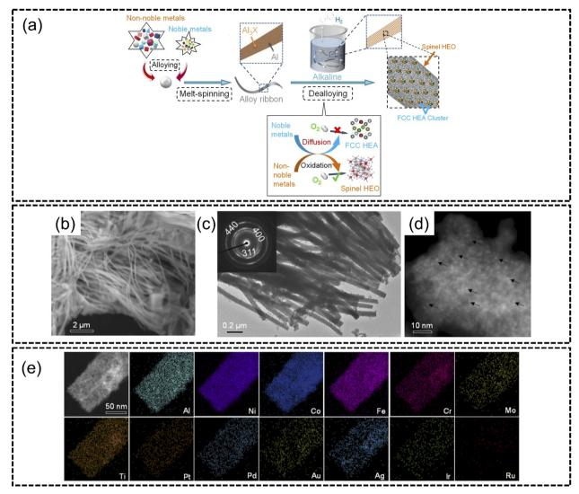
Fig. 9 Chemical dealloying synthesis from the work of Jin et al., (a) schematic illustrations of the two-step alloying and dealloying of PtPdAuAgCuIrRu HEA on (AlNiCoFeCrMoTi)<sub>3</sub>O<sub>4</sub> HEO, images of HEA cluster@HEO taken using (b) SEM, (c) TEM, (d) HAADF-STEM, and (e) STEM-EDX elemental mappings of the HEA cluster@HEO. The scale is 50 nm. Reproduced with permission.<sup>120</sup> Copyright Royal Society of Chemistry 2022
