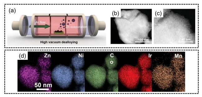
Fig. 10 Vapour phase dealloying from the work of Kwon *et al.* (a) Schematic illustration of selective Zn dealloying *via* the VPD process, and (b) and (c) STEM images, and (d) STEM-EDX elemental mapping of ZnNiCoIrMn. The scale is 50 nm. Reproduced with permission.<sup>124</sup> Copyright Wiley-VCH GmbH 2023.
