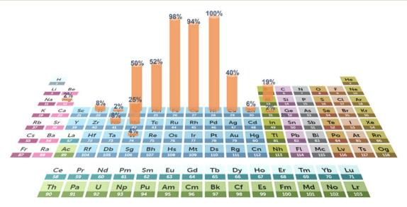
Fig. 2 Addition frequency of various elements of HEAs for HER and OER electrocatalysts from recent research. (The periodic table is from the Royal Society of Chemistry<sup>107</sup>).
