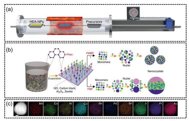
Fig. 6 FMBP synthesis from the work of Gao et al., (a) illustration of the FMBP experimental setup to synthesize HEA NPs from precursors, (b) schematics for the synthesis of HEA NPs which are homogeneous when synthesized via FMBP, and phase-separated when synthesized via fixed bed pyrolysis (FBP), and (c) STEM-EDX elemental mapping of MnCoNiCuRhPdSnIrPtAu constituents. The scale bar is 10 nm. Reproduced with permission. Copyright Springer Nature 2020.
