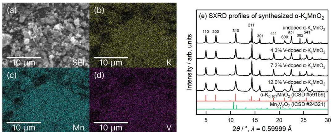
Fig. 2 (a) SEM image of 7.2% V-doped  $\alpha$ - $K_x$ MnO<sub>2</sub> and EDS elemental mapping of the corresponding area for (b) potassium, (c) manganese, and (d) vanadium. (e) SXRD profiles of undoped, 4.3% V-doped, 7.2% V-doped, and 12.0% V-doped  $\alpha$ - $K_x$ MnO<sub>2</sub>.
