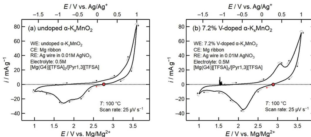
**Fig. 5** (a) Cyclic voltammogram of undoped  $\alpha$ - $K_x$ MnO<sub>2</sub> measured at a scan rate of 25  $\mu$ V s<sup>-1</sup> at 100 °C. (b) Cyclic voltammogram of 7.2% V-doped  $\alpha$ - $K_x$ MnO<sub>2</sub> measured at a scan rate of 25  $\mu$ V s<sup>-1</sup> at 100 °C.
