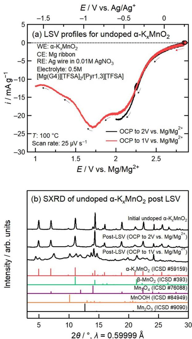
Fig. 6 (a) Linear sweep voltammograms of undoped  $\alpha$ - $K_x$ MnO<sub>2</sub> from OCP to 2 V vs. Mg/Mg<sup>2+</sup> and OCP to 1 V vs. Mg/Mg<sup>2+</sup>. (b) SXR D profiles of undoped  $\alpha$ - $K_x$ MnO<sub>2</sub> as-synthesized powder and composite electrodes containing undoped  $\alpha$ - $K_x$ MnO<sub>2</sub> following LSV from OCP to 2 V vs. Mg/Mg<sup>2+</sup> and OCP to 1 V vs. Mg/Mg<sup>2+</sup>.
