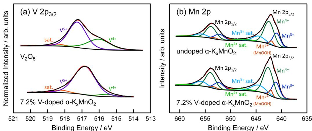
Fig. 3 X-ray photoelectron spectra: (a) V 2p<sub>3/2</sub> peak of V<sub>2</sub>O<sub>5</sub> and 7.2% V-doped  $\alpha$ - $K_x$ MnO<sub>2</sub> and (b) Mn 2p peaks of undoped  $\alpha$ - $K_x$ MnO<sub>2</sub> and 7.2% V-doped  $\alpha$ - $K_x$ MnO<sub>2</sub>.
