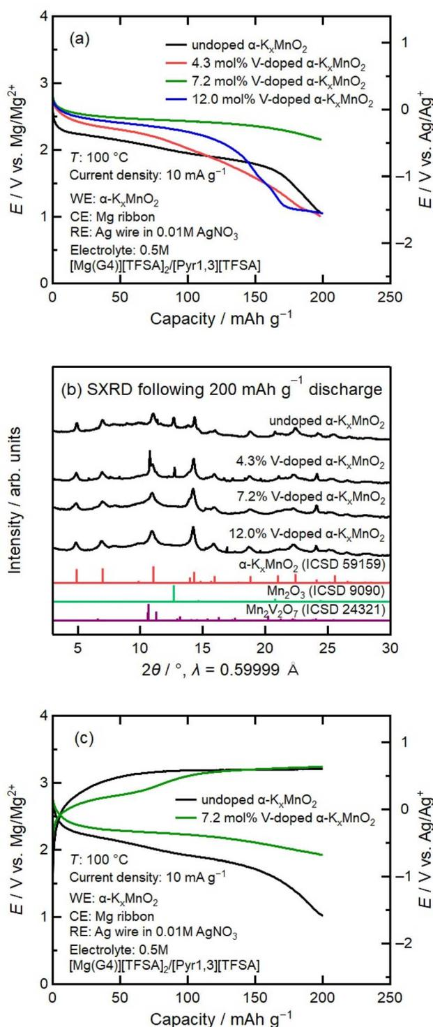
Fig. 4 (a) Constant current discharge curves of undoped and V-doped  $\alpha\text{-K}_x\text{MnO}_2$ . (b) SXR profiles of undoped and V-doped  $\alpha\text{-K}_x\text{MnO}_2$  following constant current discharge to 200 mA h g<sup>-1</sup> shown in (a). (c) Constant current discharge-charge curves of undoped and 7.2% V-doped  $\alpha\text{-K}_x\text{MnO}_2$ .
