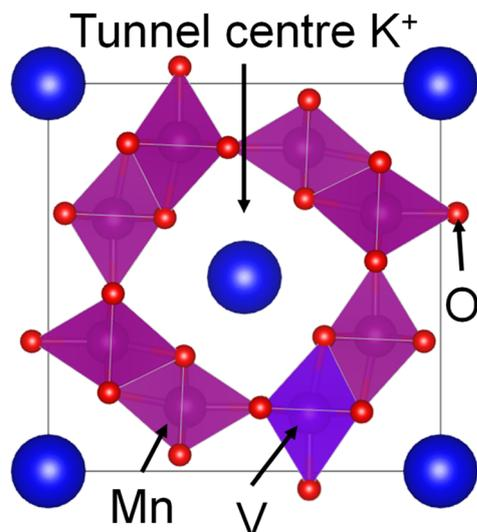
Fig. 1 Schematic diagram of potassium stabilized hollandite manganese oxide ( $\alpha\text{-K}_x\text{MnO}_2$ ) with K, Mn, O and substituted V positions labelled. VESTA 3 is used for three-dimensional visualization of the crystal.
