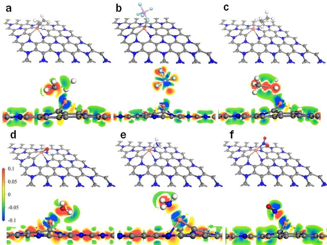
Fig. 3 Stable configurations and charge density of gas adsorbed on the Cu-C<sub>2</sub>N<sub>1</sub> monolayer: (a) Cu-C<sub>2</sub>N<sub>1</sub>-C<sub>2</sub>H<sub>4</sub>, (b) Cu-C<sub>2</sub>N<sub>1</sub>-C<sub>2</sub>H<sub>6</sub>, (c) Cu-C<sub>2</sub>N<sub>1</sub>-PF<sub>5</sub>, (d) Cu-C<sub>2</sub>N<sub>1</sub>-H<sub>2</sub>O, (e) Cu-C<sub>2</sub>N<sub>1</sub>-NH<sub>3</sub>, and (f) Cu-C<sub>2</sub>N<sub>1</sub>-NO<sub>2</sub>.
