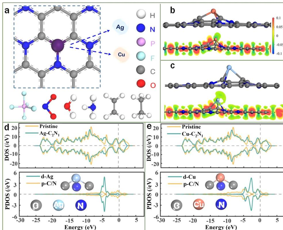
Fig. 1 (a) Structures of the Cu/Ag- $C_2N_1$  monolayer,  $PF_5$ ,  $NO_2$ ,  $NH_3$ ,  $H_2O$ ,  $C_2H_4$ , and  $C_2H_6$ . (b and c) Stable structure and charge density distribution of (b) Cu- $C_2N_1$  and (c) Ag- $C_2N_1$ . (d and e) DOS and PDOS of (d) Ag- $C_2N_1$  and (e) Cu- $C_2N_1$ . Densities are displayed with an isosurface and the interval of isovalues is between  $-0.1$  and  $0.1 \text{ e} \text{ \AA}^{-3}$ .
