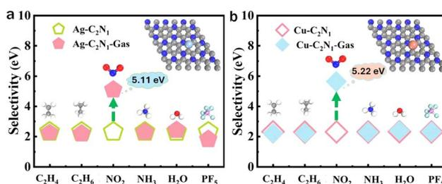
Fig. 5 Selectivity of gases on the (a) Ag-C<sub>2</sub>N<sub>1</sub> and (b) Cu-C<sub>2</sub>N<sub>1</sub> monolayers.
