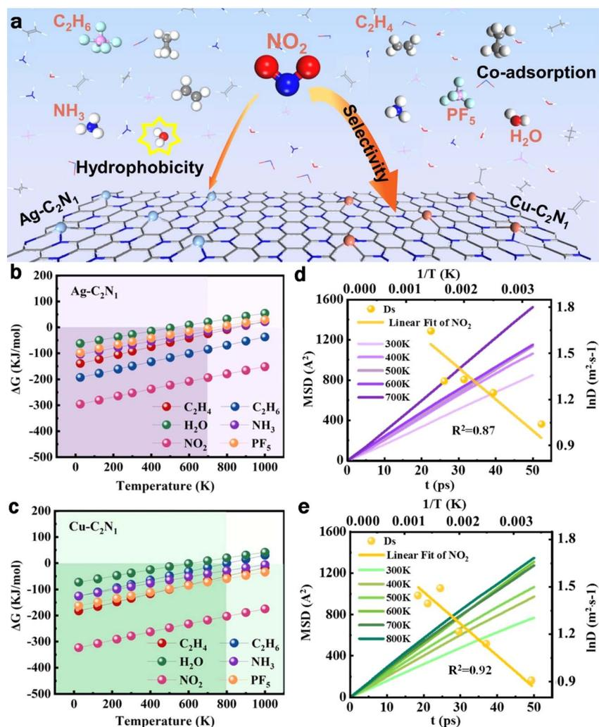
Fig. 6 (a) Schematic diagram of the high selectivity and hydrophobicity of Cu/Ag-C<sub>2</sub>N<sub>1</sub>. The Gibbs free energy of the six gases on (b) Ag-C<sub>2</sub>N<sub>1</sub> and (c) Cu-C<sub>2</sub>N<sub>1</sub> as a function of temperature. Gas diffusion and mean-squared displacement on (d) Ag-C<sub>2</sub>N<sub>1</sub> and (e) Cu-C<sub>2</sub>N<sub>1</sub> at different temperatures.
