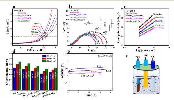
Fig. 3 (a) LSV polarization results of ZIF-8, NC(ZnO),  $Ru_{0.75}$ @NC(ZnO),  $Ru_{1.75}$ @NC(ZnO) and  $Ru_{3}$ @NC(ZnO); (b) EIS outcomes; the inset shows the equivalent circuit diagram; (c) iR drop free Tafel slope; (d) overpotential measured at different current densities; (e) long term-static stability at an applied current density of 10 mA cm<sup>-2</sup>; (f) cell representation of the three-electrode setup used for OER performance.
