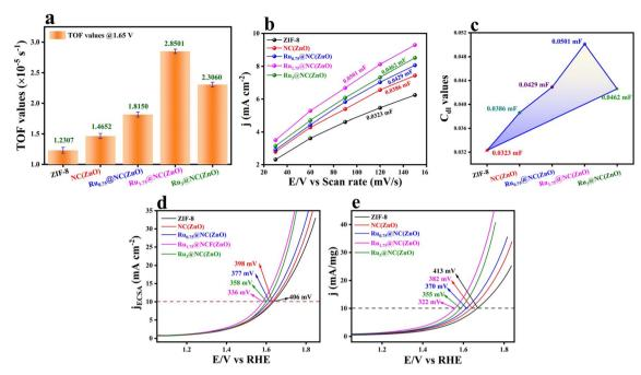
Fig. 4 (a) TOF values of ZIF-8, NC(ZnO), Ru<sub>0.75</sub>@NC(ZnO), Ru<sub>1.75</sub>@NC(ZnO)and Ru<sub>3</sub>@NC(ZnO); (b) C<sub>dl</sub> values measured from the CV curves; (c) comparison of the C<sub>dl</sub> values; (d) ECSA normalized (specific activity) LSV polarization results; (e) mass dependent activity of all the catalysts.
