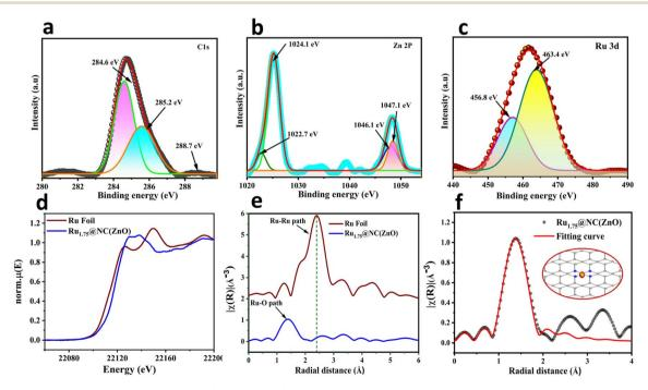
Fig. 2 High-resolution XPS spectra of (a) C 1s, (b) Zn 2p, and (c) Ru 3d, (d) XANES spectra of the sample measured at Ru K edge, (e) Fourier transformed EXAFS spectra of the sample measured at Ru K edge, and (f) EXAFS fitting curve for Ru<sub>1.75</sub>@NC(ZnO).
