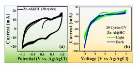
Fig. 4 (a) 20 Cycles CV under ideal operating conditions, (b) 20 cycles CV for Zn-Al@HC (real environmental conditions; both UV illuminated and dark systems).
