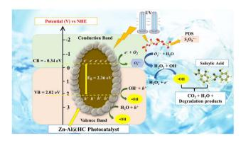
Fig. 9 Proposed photocatalytic mechanism of Zn-Al@HC for reactive radical generation, PDS activation, and SA degradation.
