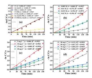
Fig. 6 (a) Photocatalytic degradation of SA and kinetics involved under different (b) PDS dosages, (c) Zn–Al@HC dosages, and (d) pollutant concentrations. (pH $_0$  of 7.0, temperature of 27 °C, Zn–Al@HC of 10 mg  $L^{-1}$ , UV irradiation of 11  $\mu W$  cm $^{-2}$ , SA concentration of 50 mg  $L^{-1}$ , and PDS of 0.01 M.)
