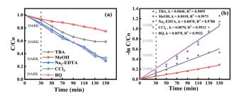
Fig. 7 (a) Scavenging effect of TBA, MeOH, Na<sub>2</sub>-EDTA, CCl<sub>4</sub>, and BQ on SA decay and (b) kinetics in the UV/PDS/Zn-Al@HC system.
