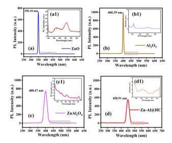
Fig. 5 PL spectra and sub-spectra of (a and a1) pure ZnO, (b and b1) pure Al<sub>2</sub>O<sub>3</sub>, (c and c1) co-precipitated ZnAl<sub>2</sub>O<sub>4</sub>, (d and d1) and assynthesized Zn-Al@HC photocatalyst.
