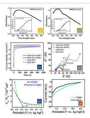
Fig. 3 (a and b) UV-DRS of pristine HC and Zn-Al@HC, (c) chronoamperometric analysis of HC and Zn-Al@HC (UV illuminated and dark system), (d) Nyquist plot for HC and Zn-Al@HC under UV and dark conditions, and (e) Mott-Schottky plot under UV light, (f) LSV curves under UV illuminated and dark conditions.
