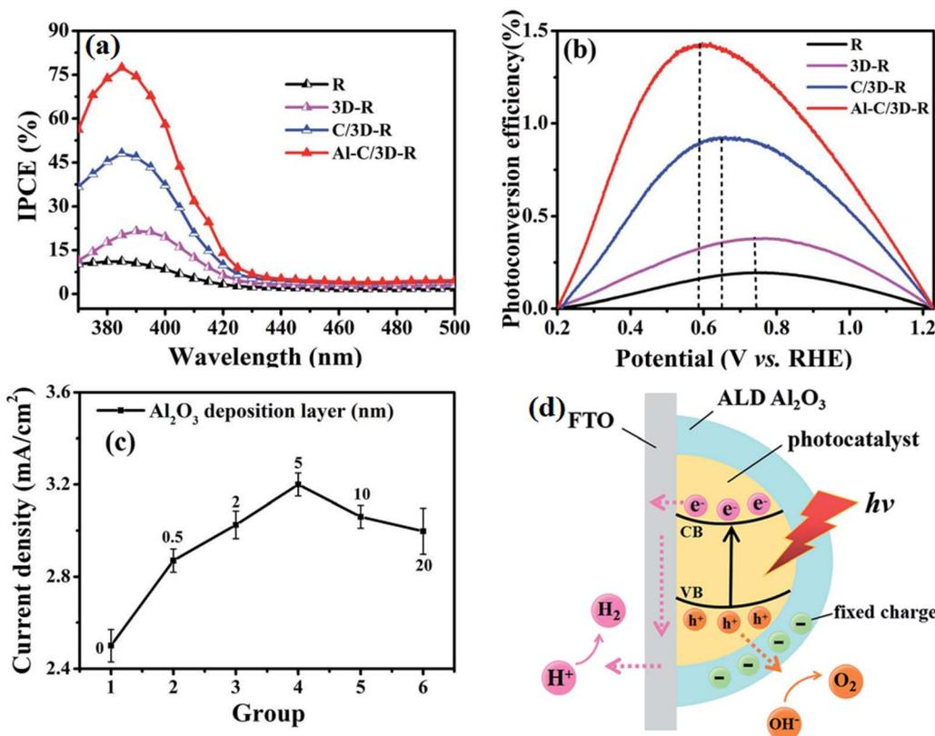
Fig. 17 (a) IPCE spectra and (b) calculated solar-to-hydrogen (STH) efficiencies of the samples. (c) Line chart measured at 1.23 V vs. RHE of thickness of Al<sub>2</sub>O<sub>3</sub> layer. (d) Mechanism model for the role of Al<sub>2</sub>O<sub>3</sub> coating in the separation of electron–hole pairs. Reproduced with permission from ref. 56. Copyright 2018, the Royal Society of Chemistry.
