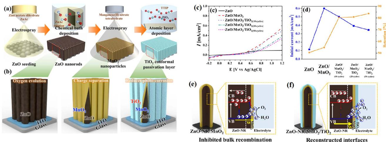
Fig. 15 (a) Schematic of the fabrication of ZnO/MnO<sub>2</sub>/TiO<sub>2</sub> nanorods, (b) illustration of the effect of each coated layer, (c) and (d) are respectively photocurrent density and stability of the samples, and effects of (e) MnO<sub>2</sub> in promoting charge separation and (f) TiO<sub>2</sub> as a passivation layer. Reproduced with permission from ref. 91. Copyright 2020, Elsevier.
